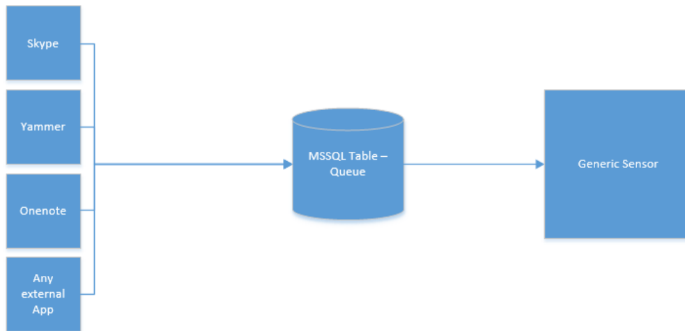
Figure 11: Workflow of the and architecture of the Generic Sensor that is implemented.
