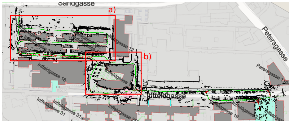
(a) Overview of the official map with the overlaying pose-graph. The laser scans are colored in black. The red rectangle a) shows the extracted close up related to Figure 7.7b and b) relates to Figure 7.7c.
