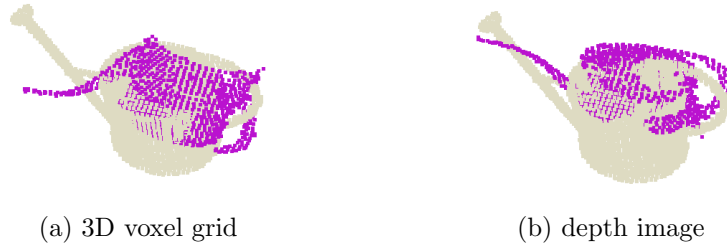
Figure 45: Alignment of a model (grey) to a scan (purple) using the voxel grid and the depth image representation.
