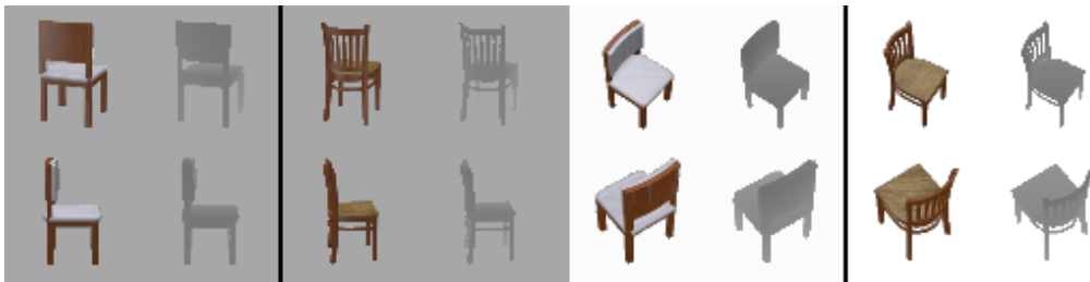
Figure 51: Retrieval results using the trained network on a synthetically generated test dataset. The first columns show the query pose and the second columns show the best matching pose of the template object respectively. (for more results see Appendix)
