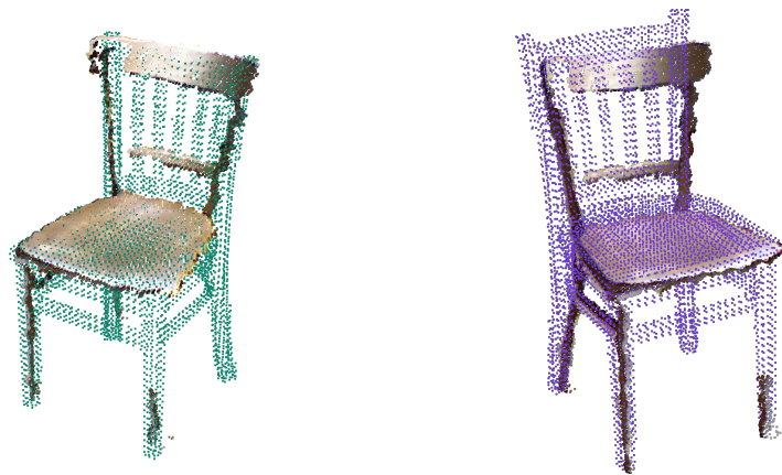
(a) Alignment using the voxel image approach and a known upper axis.
