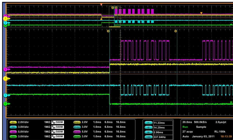
Figure 9.21 : Modulated Start sequence after reset on the CLMCS supply
