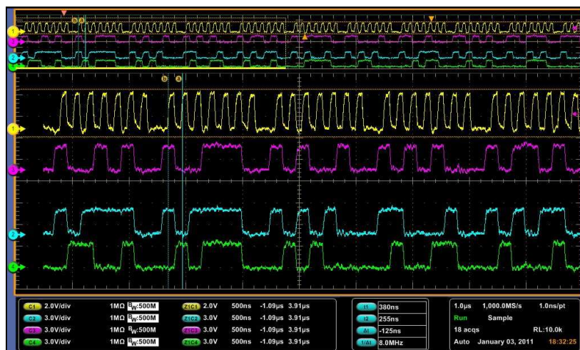
Figure 9.7 : Measured digital output signals from the CLMCS
