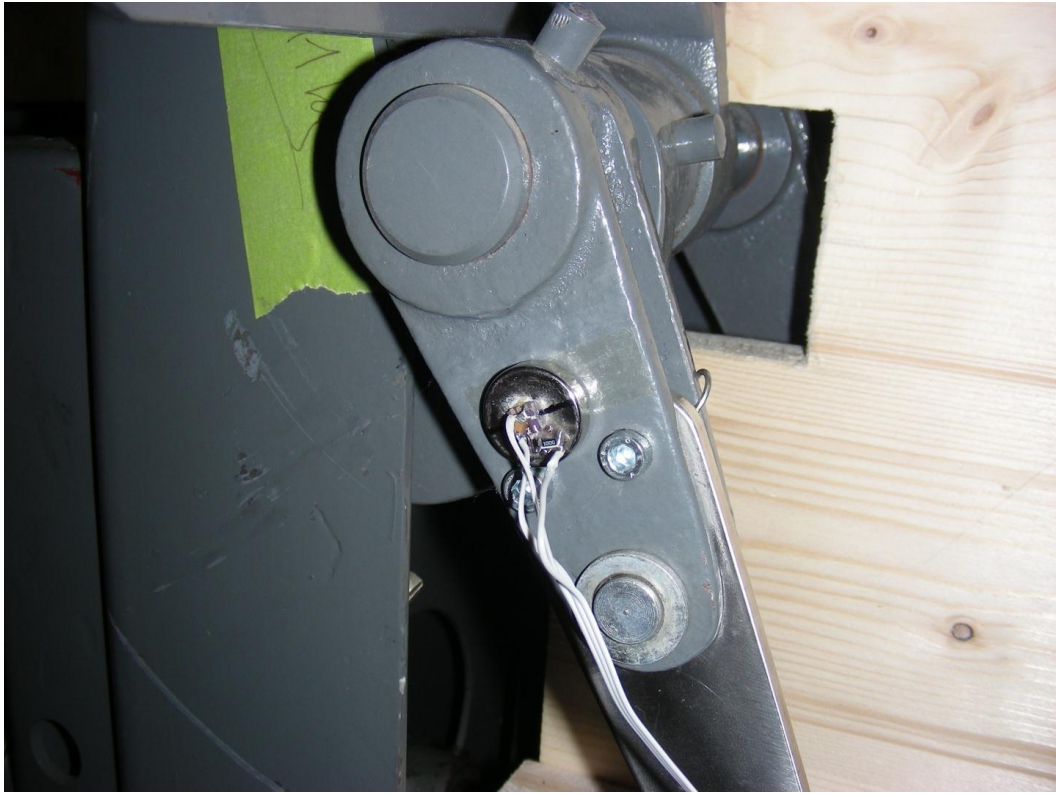
Figure 44: Mounted sensor using a thin double-sided adhesive tape between magnet and MCVB.
