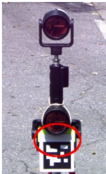
Figure 5-5: Auxiliary prism partly shadowing the fiducial marker at a distance of 4.6 m
