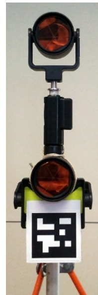
Figure 1-2: Prototype of the modified reflector pole
