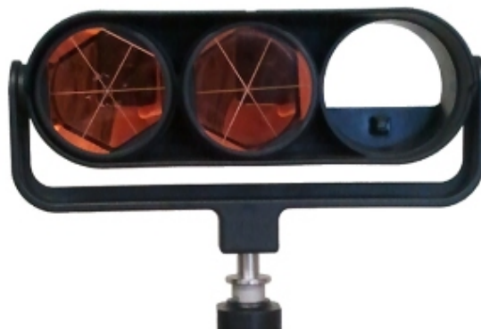
Figure 3-27: Leica GPH3 triple prism holder with two prisms mounted next to each other (73.2 mm separation between the prism centres)
