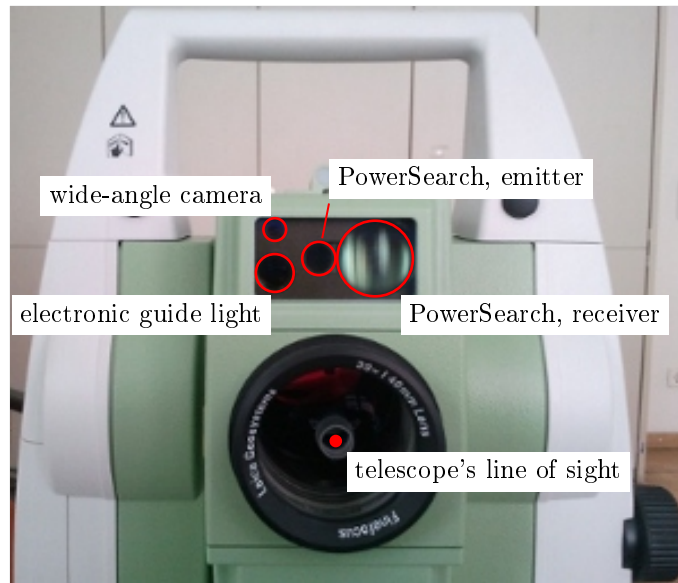
Figure 4-1: Offset between the centres of the telescope and the wide-angle camera
