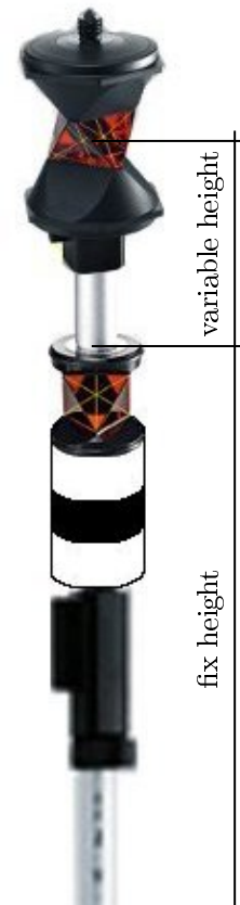
Figure 7-1: Design study of a modified reflector pole
