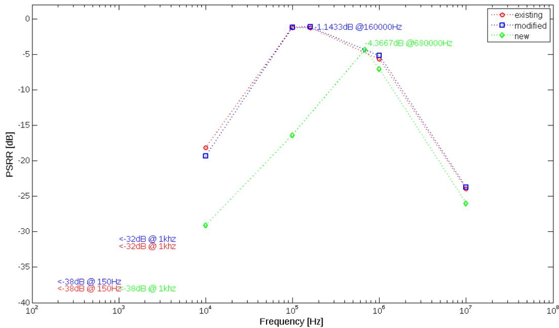
Figure 7.14: PSRR of the regulators, at minimal dropout voltage.
