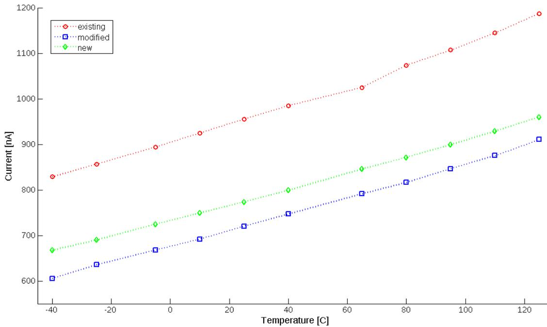
Figure 7.2: Measured current consumption of the regulators versus temperature
