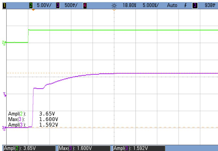
Figure 7.7: New regulator: Overshoot of the output voltage due to a fast rising supply voltage.
