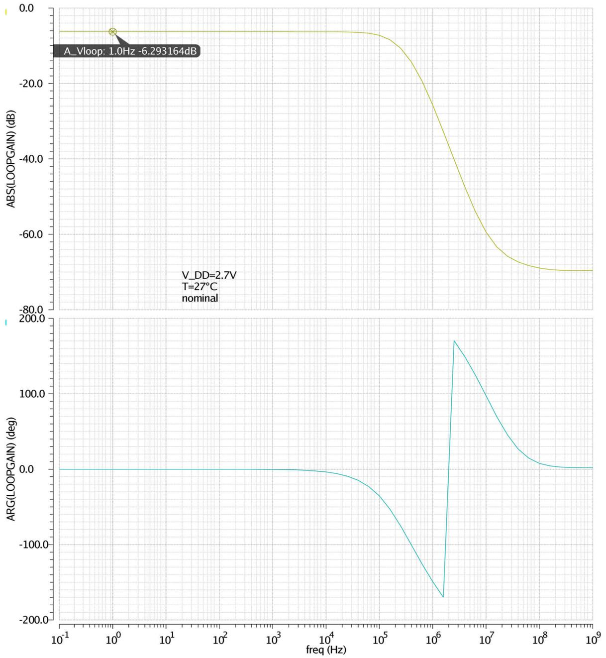
Figure 4.9: Loop gain of the bias regulation.
