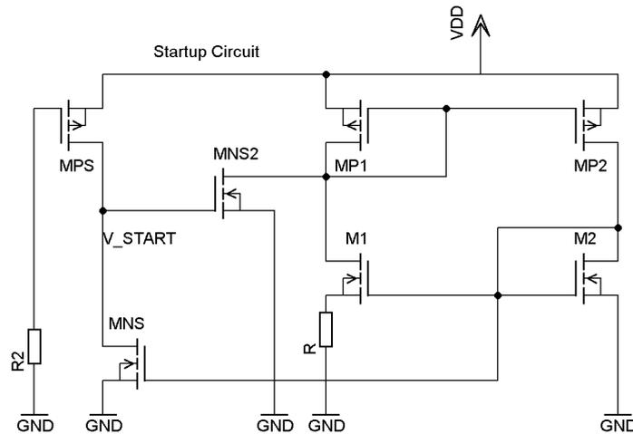
Figure 4.5: Schematic diagram of bias start-up circuit.
