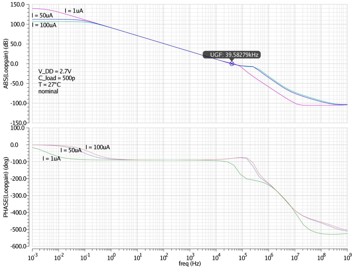
Figure 6.5: Bode plot of the loop gain.
