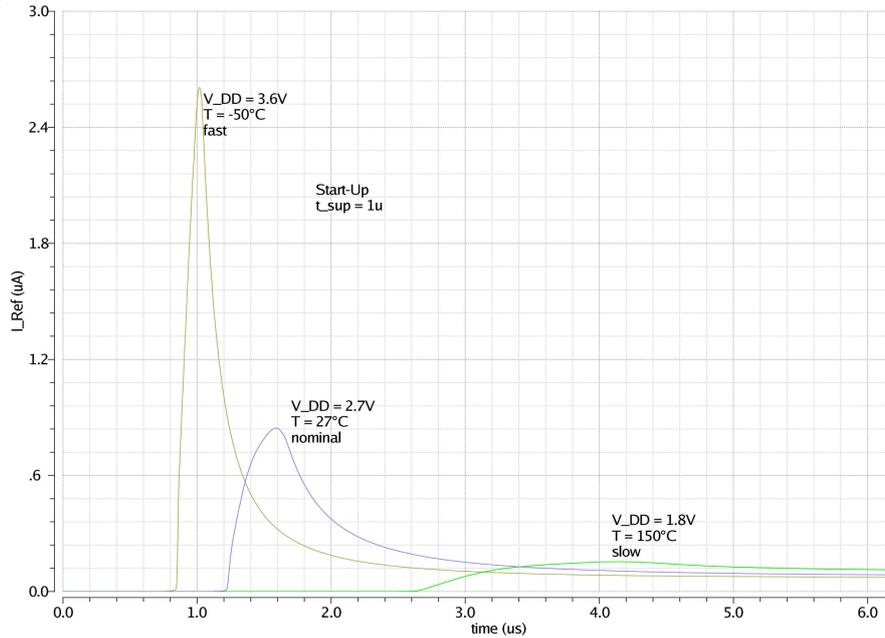
Figure 4.8: Start-up of the bias circuit.
