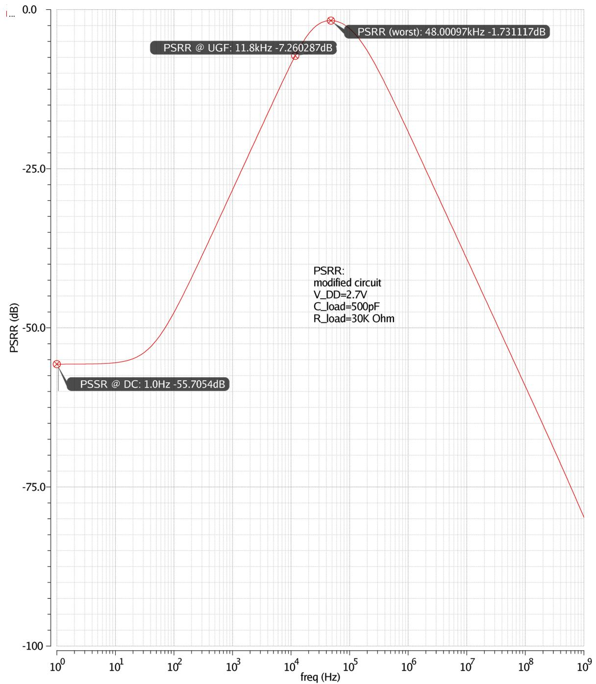
Figure 5.6: Plot of the improved circuit's PSRR over frequency.
