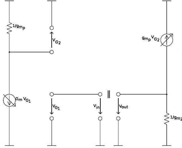
Figure 4.3: Small signal equivalent circuit of the beta multiplier.
