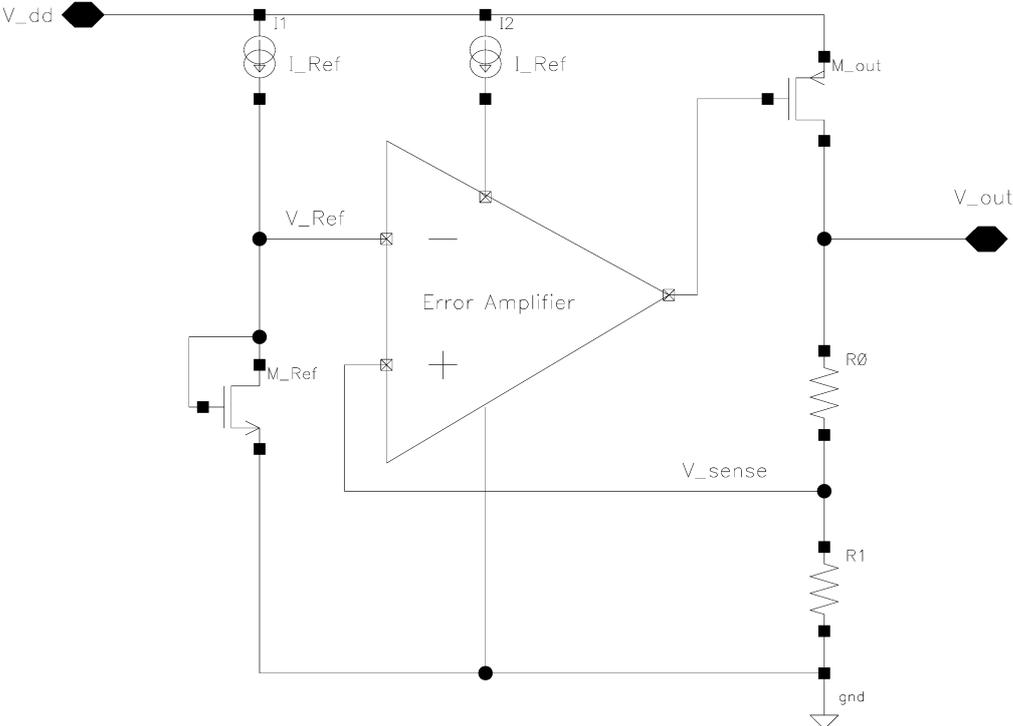
Figure 2.1: Topology of the regulator circuit
