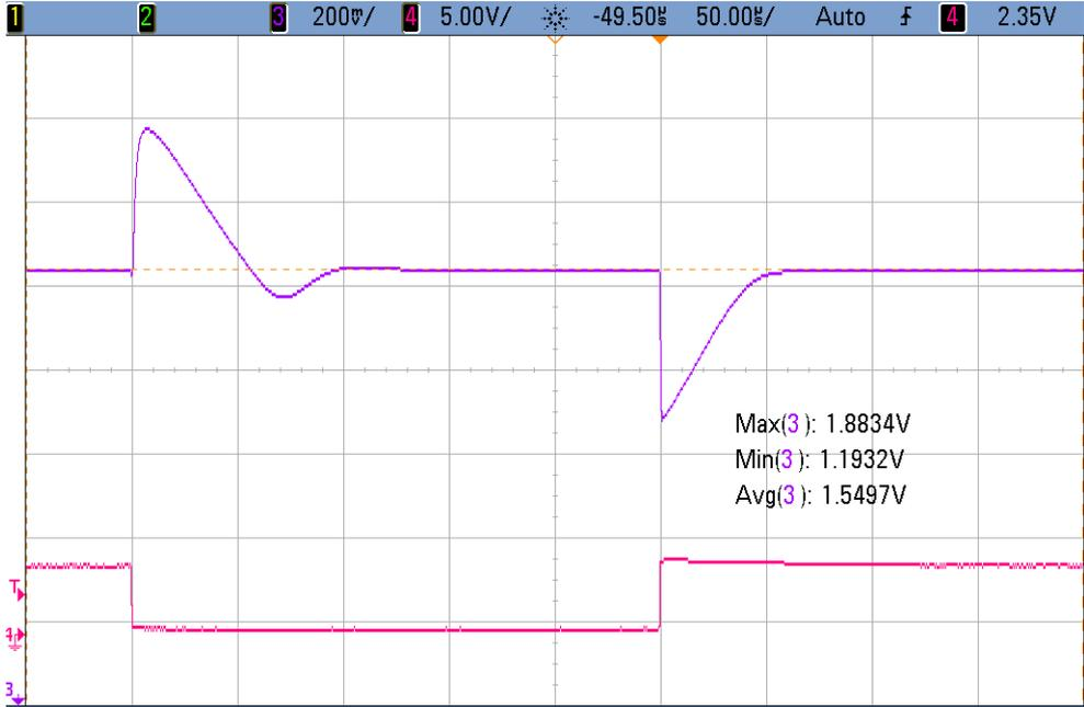
Figure 7.9: Modified regulator: Response of the output voltage to a large load step.
