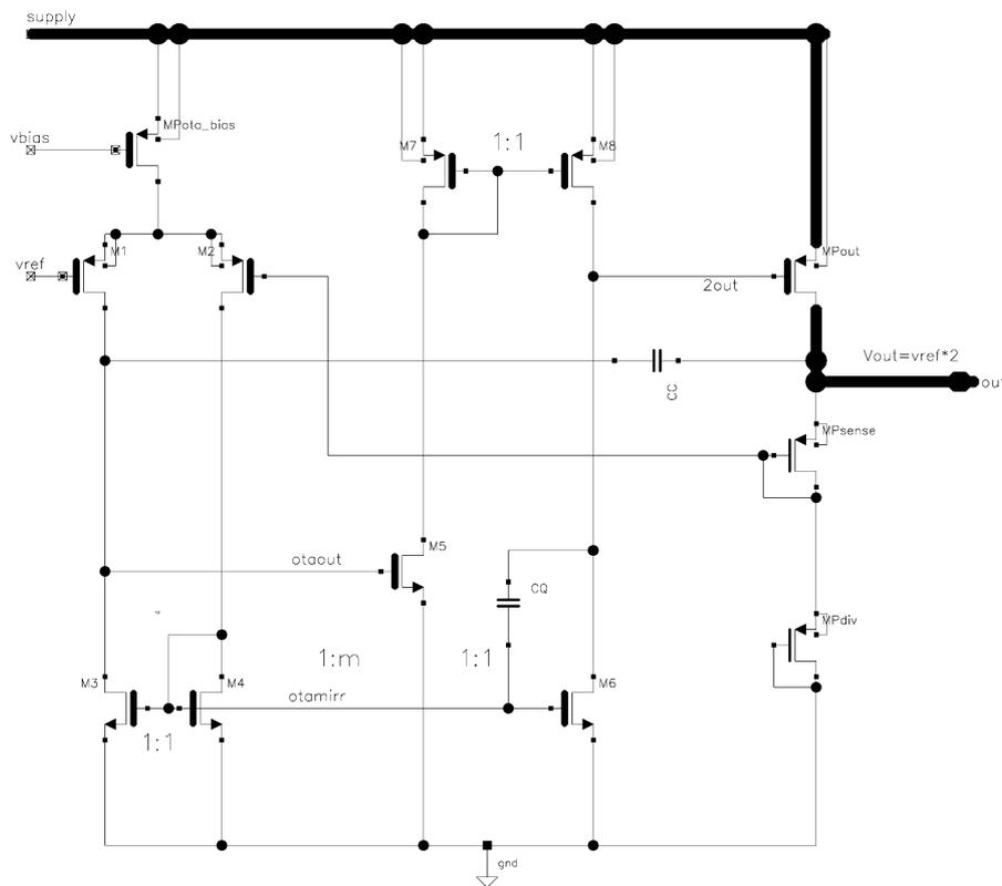
Figure 6.1: Schematic of regulator circuit proposed by Lau, Mok, and Leung [16].
