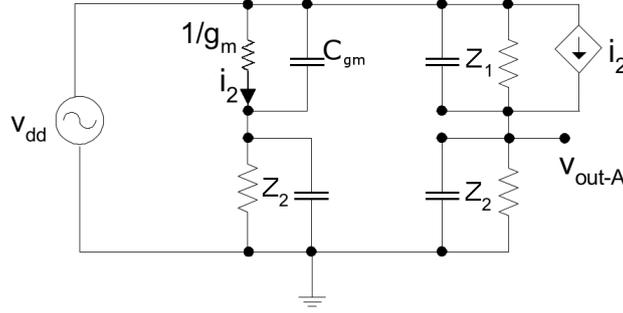
Figure 3.7: Extended OTA model, derived from Gupta, Rincon-Mora, and Raha [10].
