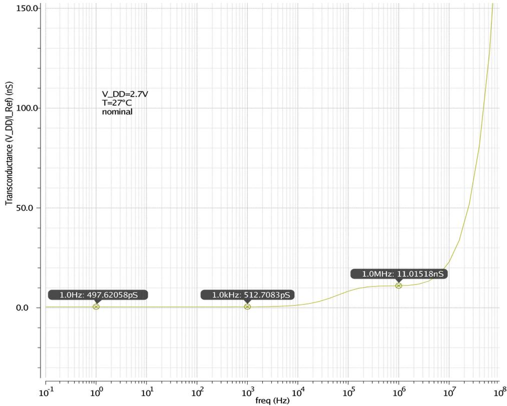
Figure 4.10: Power supply ripple dependence of the bias circuit: Transconductance from  $V_{DD}$  to  $I_{Ref}$ .
