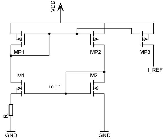
Figure 4.1: Schematic diagram of the bias circuit.
