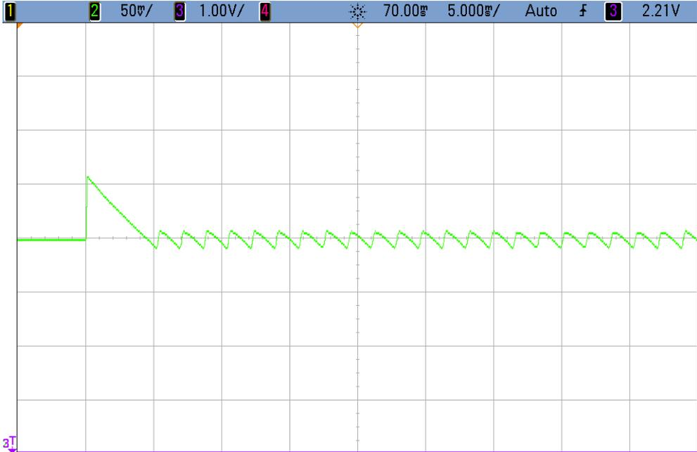
Figure 7.16: Existing regulator: Small signal load step response, no load condition.
