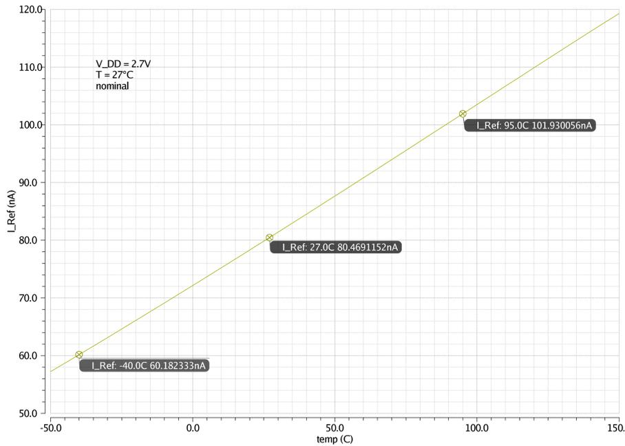
Figure 4.7: Temperature plot of the bias current.
