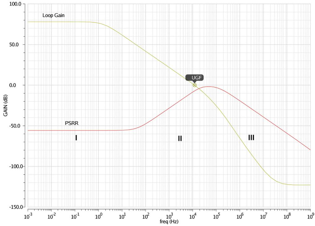
Figure 3.5: Relationship between loop gain and PSRR.
