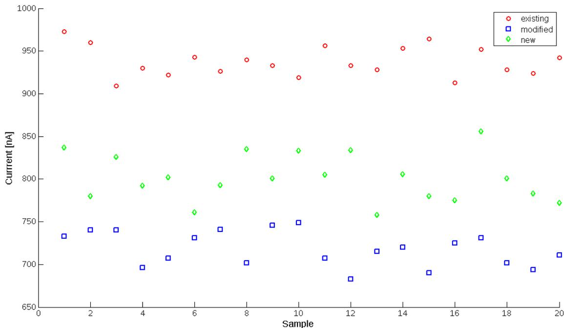
Figure 7.4: Measured current consumption of all samples at 25 °C
