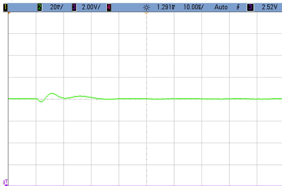
Figure 7.13: New regulator: Small signal load step response.
