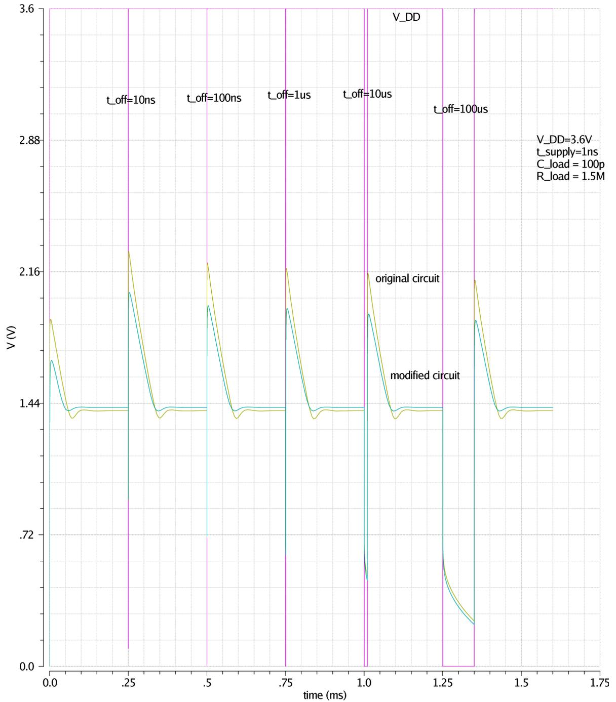
Figure 5.4: Transient response of the regulator to supply voltage variations.
