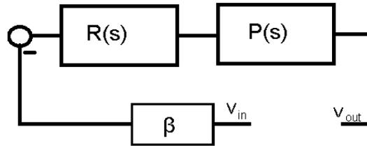
Figure 3.4: Configuration for measuring the Bode plot of the loop gain.
