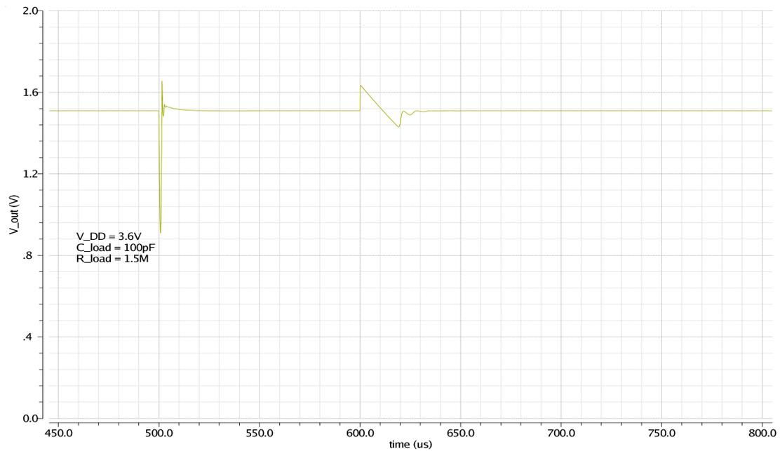
Figure 6.7: Transient response of the regulator to load changes.
