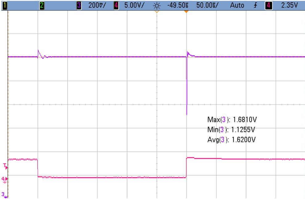
Figure 7.10: New regulator: Response of the output voltage to a large load step.
