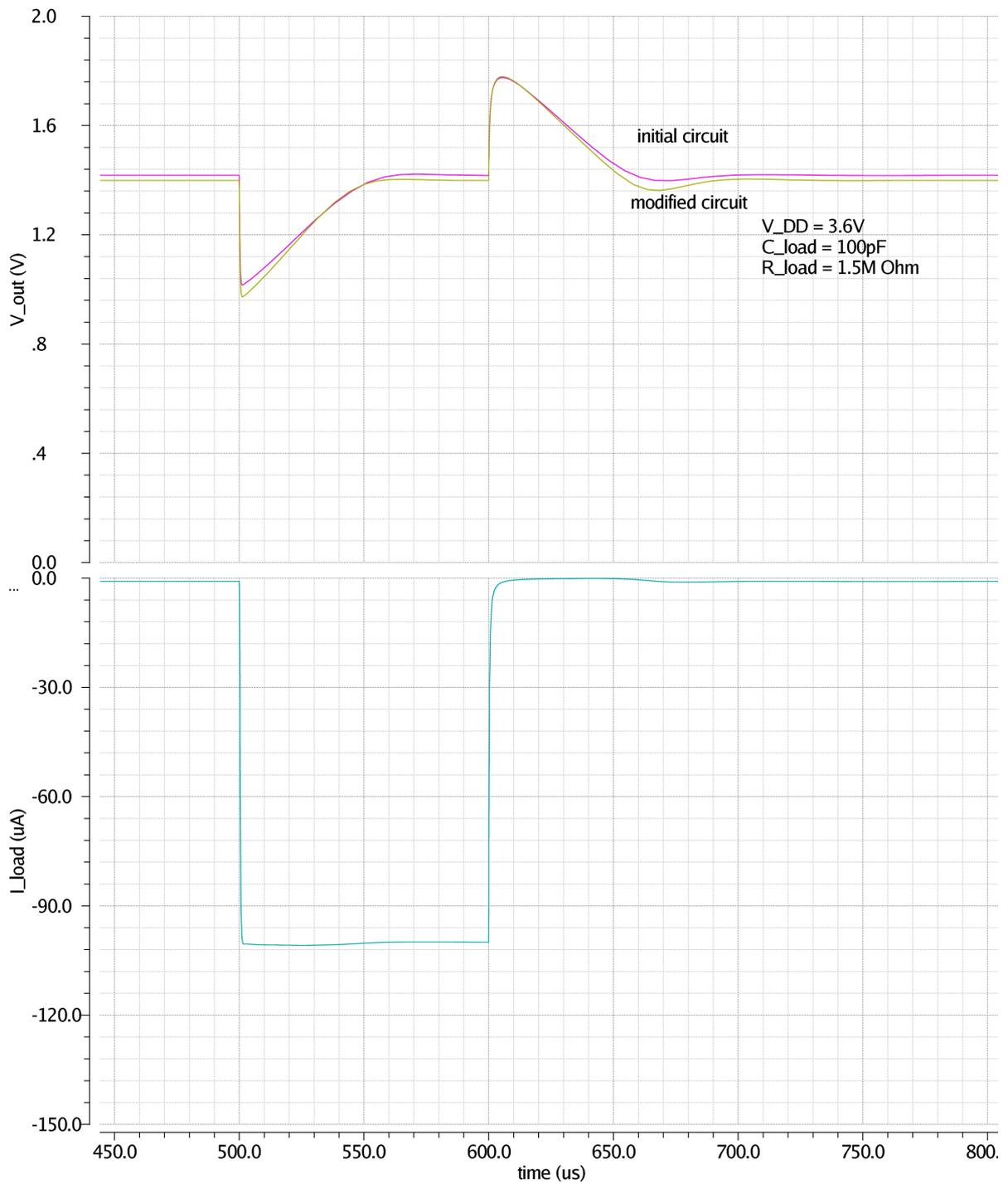
Figure 5.5: Transient response of the regulator to load changes.
