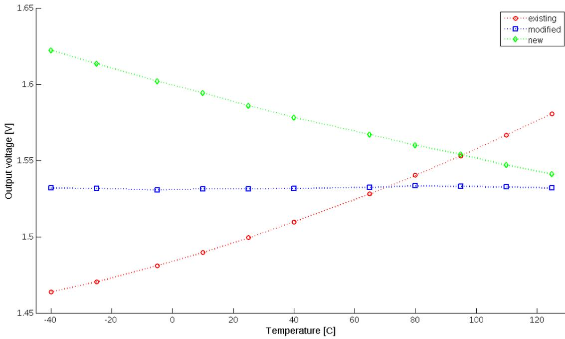
Figure 7.1: Measured output voltage of the regulators versus temperature
