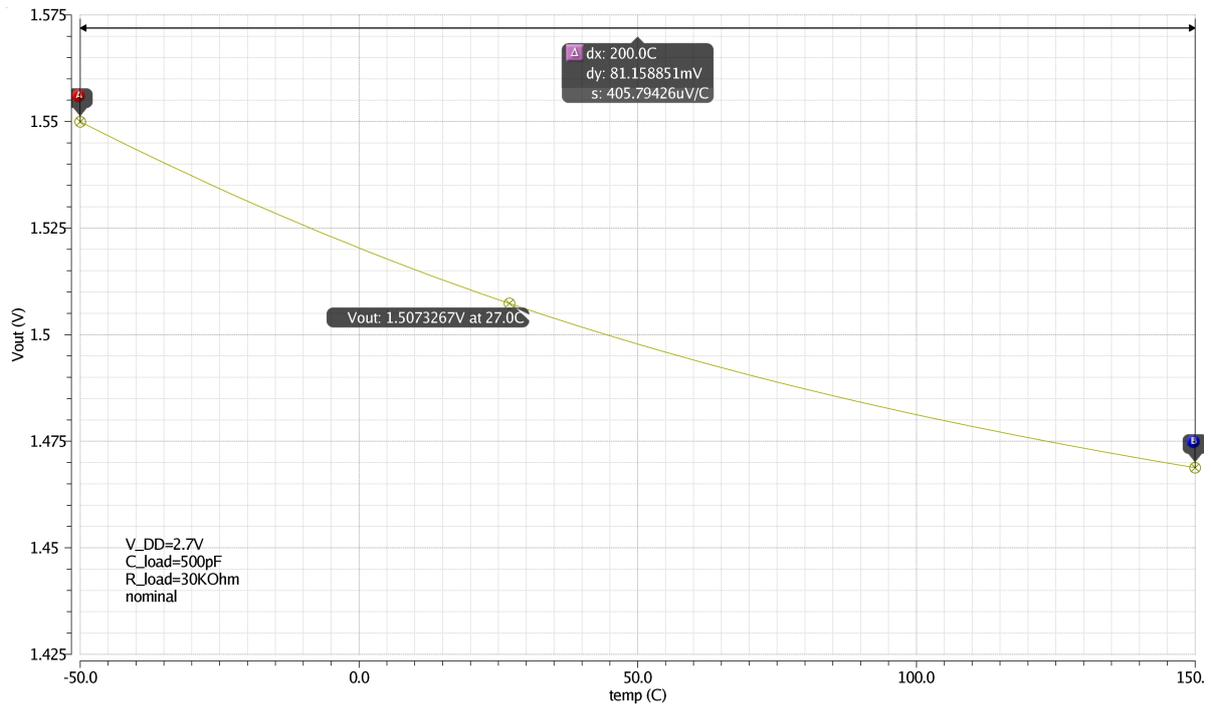
Figure 6.4: Output voltage of the regulator plotted versus temperature.
