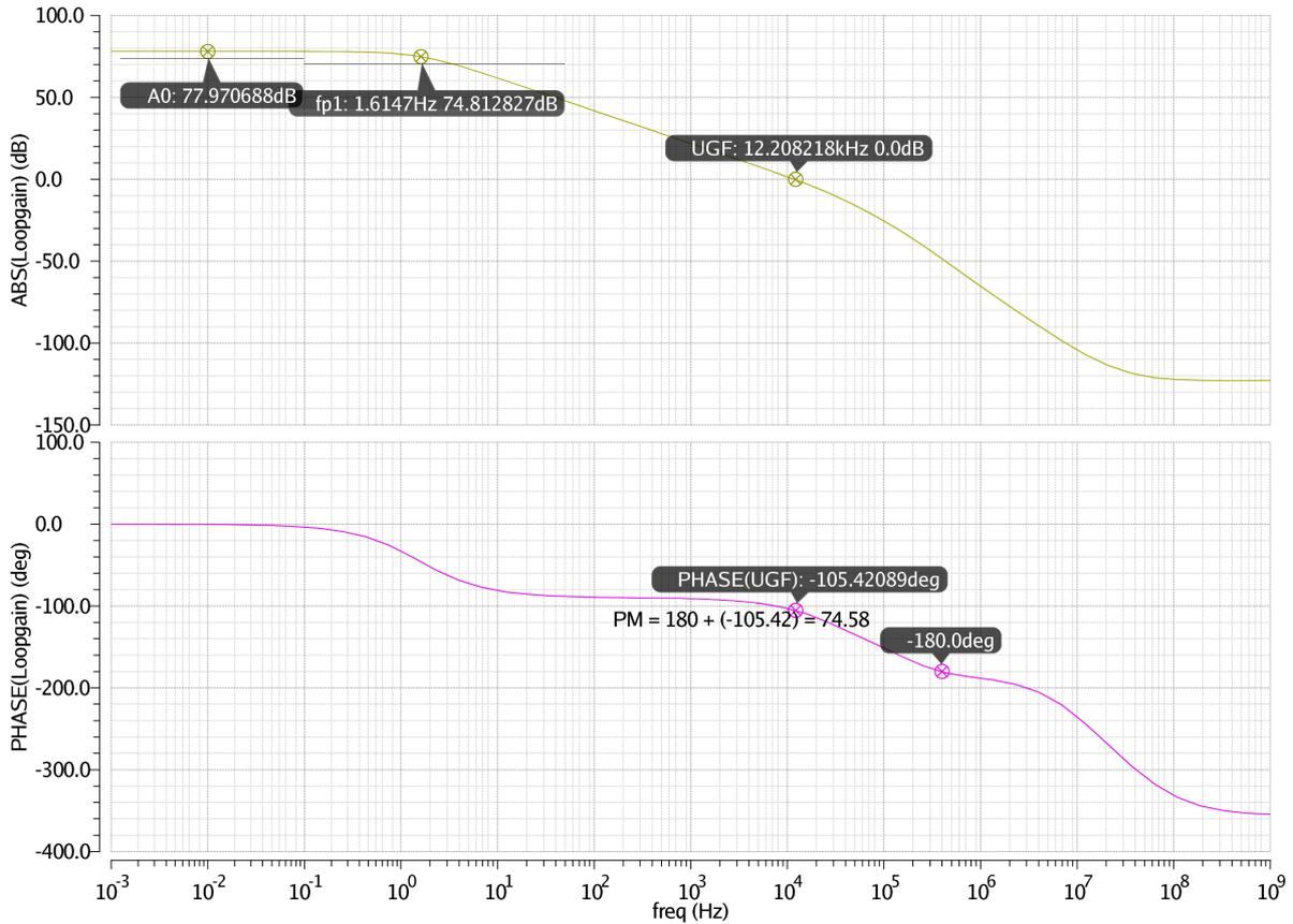
Figure 3.3: Typical Bode plot of a loop gain with dominant pole.
