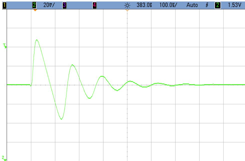
Figure 7.11: Existing regulator: Small signal load step response.
