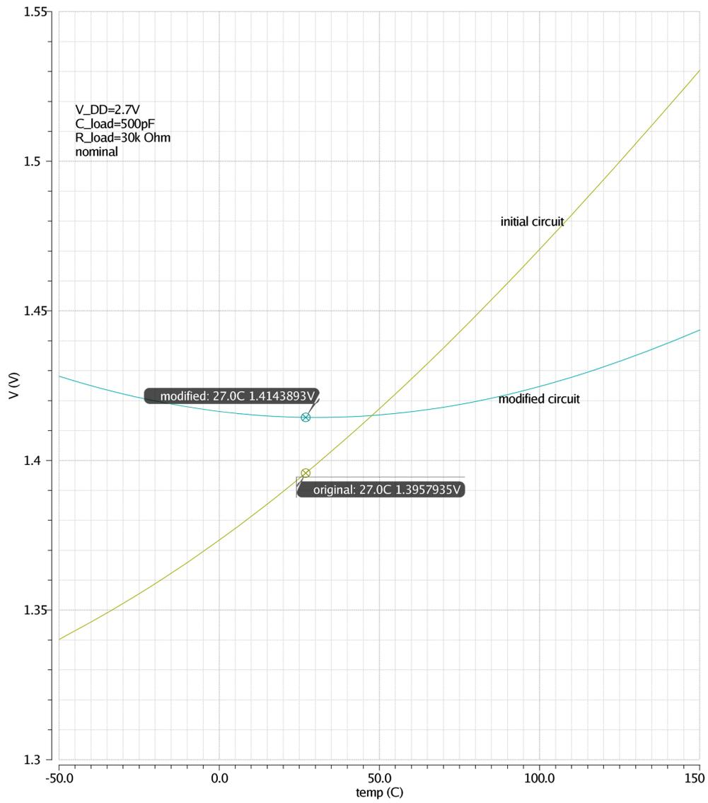
Figure 5.3: Output voltage of the regulator plotted over temperature.
