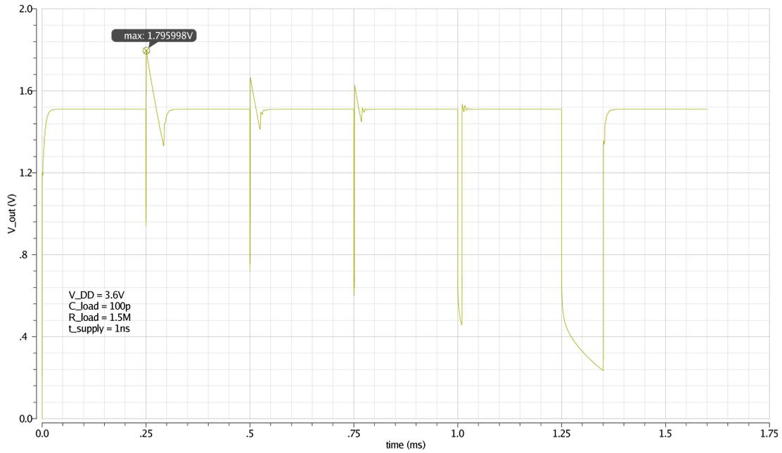
Figure 6.6: Transient response of the regulator to supply voltage variations.
