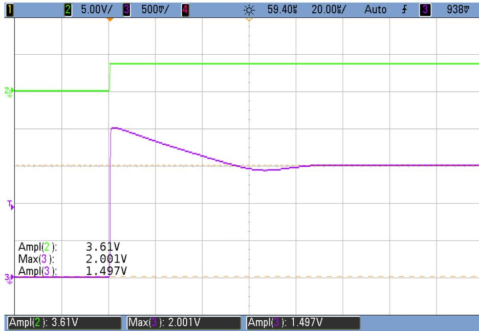
Figure 7.5: Existing regulator: Overshoot of the output voltage due to a fast rising supply voltage.
