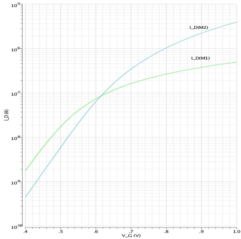
Figure 4.2: Drain current plotted versus gate voltage of M1 and M2.
