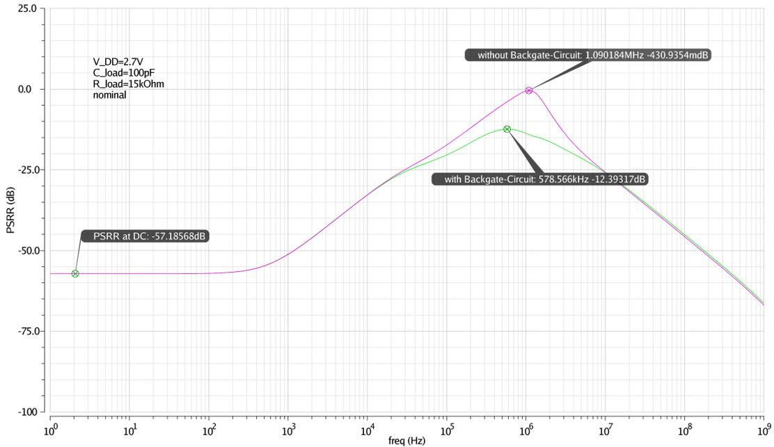
Figure 6.8: Plot of the PSRR versus frequency for the regulator with and without back gate circuit.
