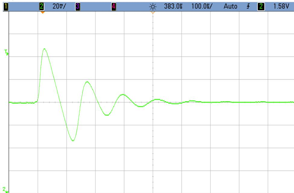
Figure 7.12: Modified regulator: Small signal load step response.
