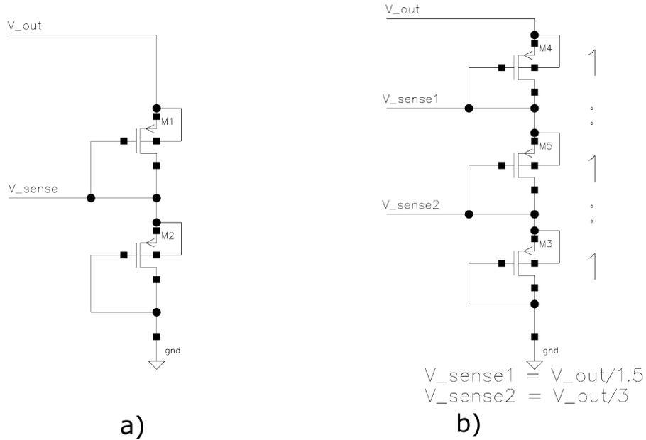
Figure 3.1: Simplified diagram of a MOSFET voltage divider.
