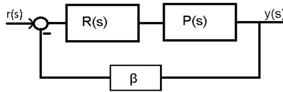
Figure 3.2: Simple model of the control system's topology.
