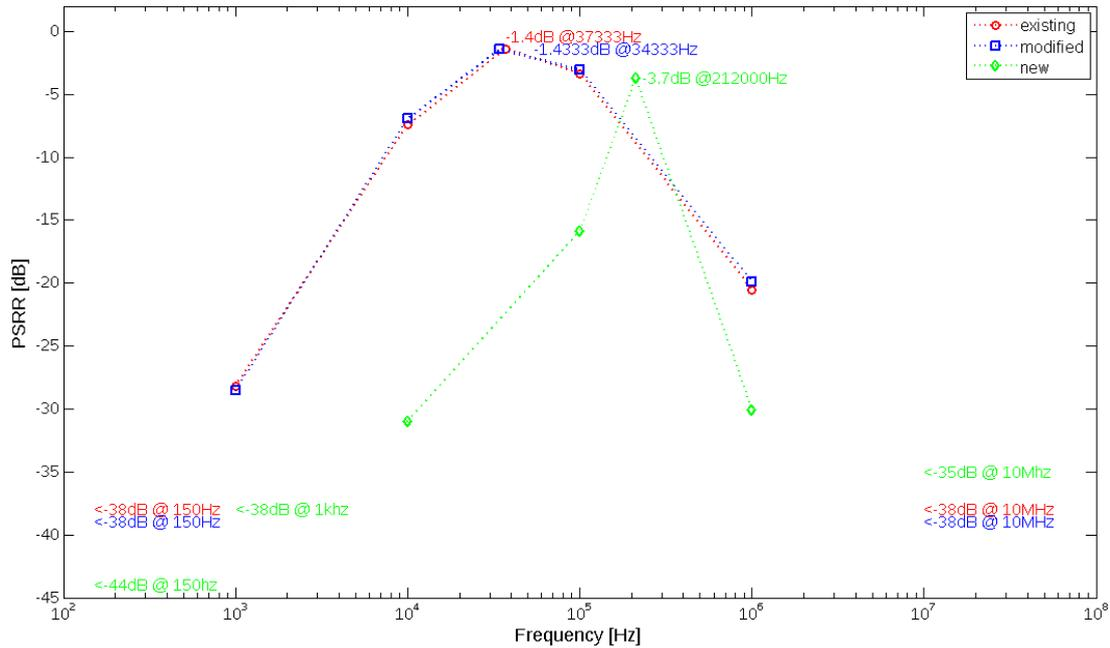
Figure 7.15: PSRR of the regulators, at typical conditions
