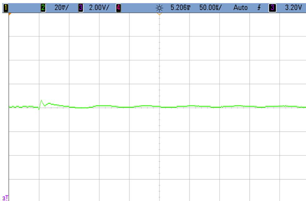
Figure 7.18: New regulator: Small signal load step response, no load condition.
