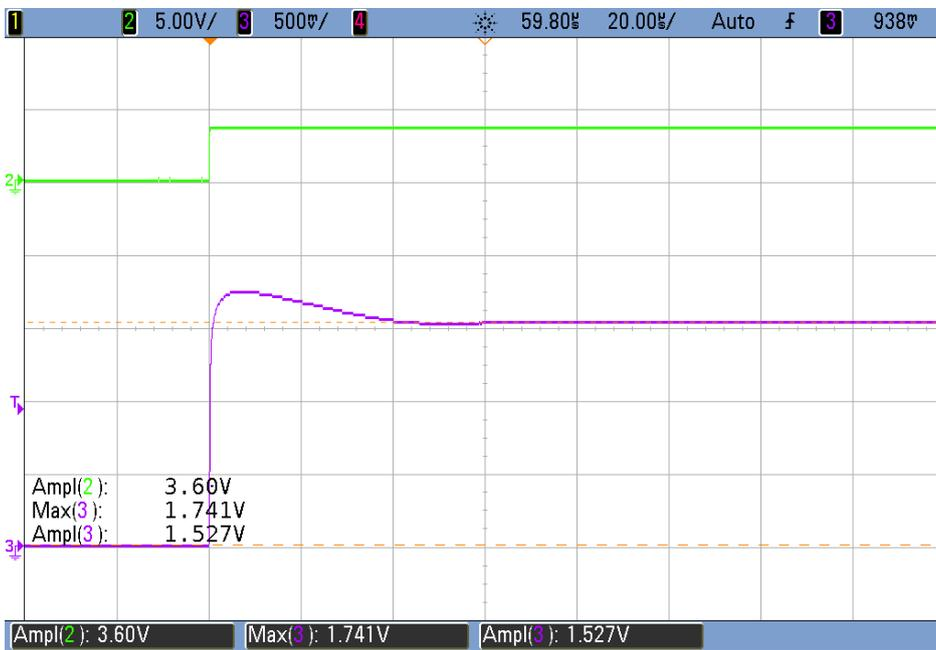
Figure 7.6: Modified regulator: Overshoot of the output voltage due to a fast rising supply voltage.
