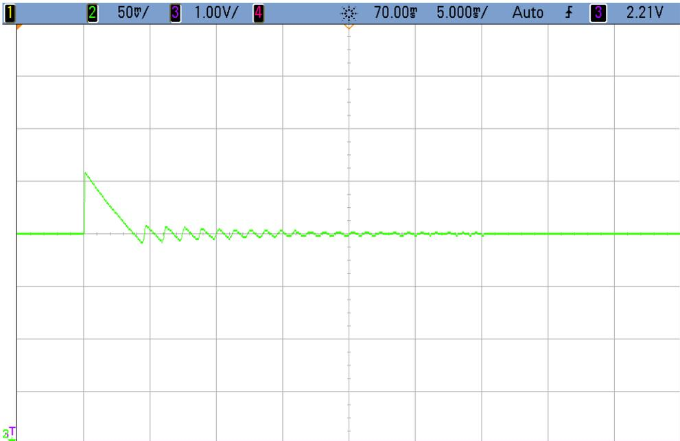
Figure 7.17: Modified regulator: Small signal load step response, no load condition.
