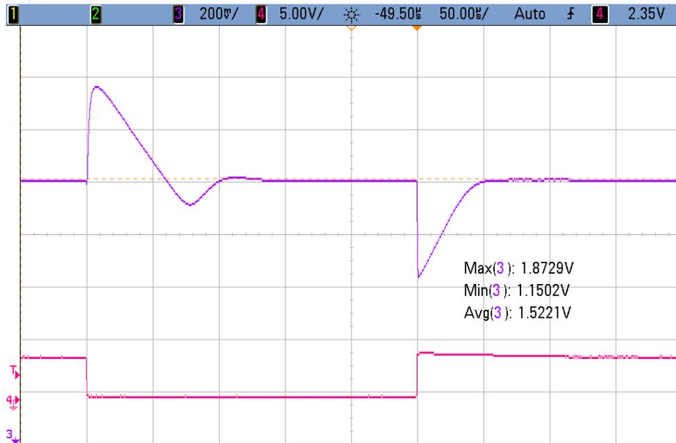
Figure 7.8: Existing regulator: Response of the output voltage to a large load step.
