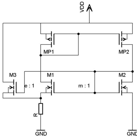
Figure 4.4: Schematic diagram of the beta multiplier circuit with bypass transistor.
