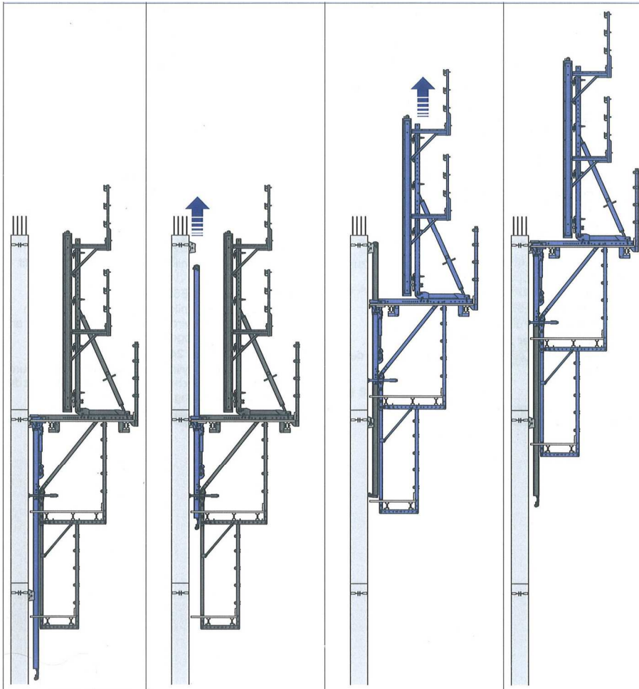
Fig. 5.6 Functional principle of crane independent jumpform of DOKA 72
