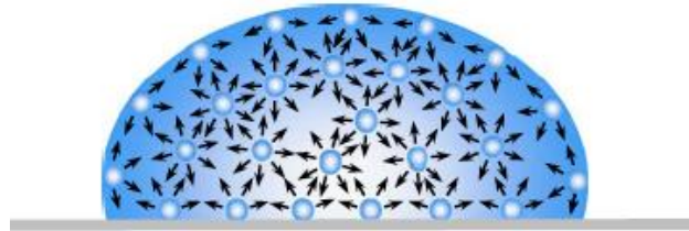
Figure 17: Interactions in a liquid droplet 38
