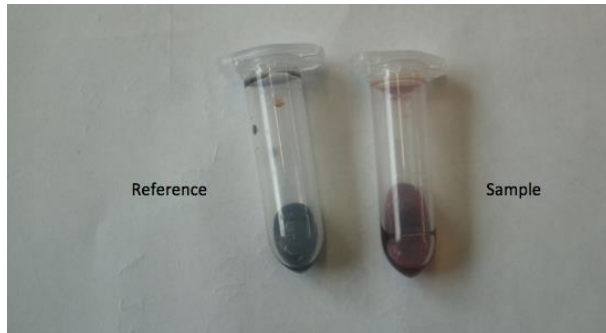
Figure 55: Ninhydrin test of APTES treated PDMS in an eppi
