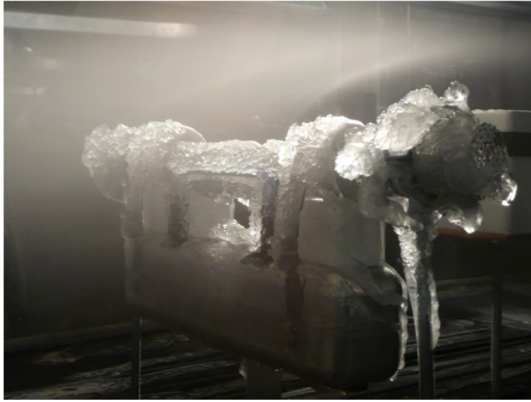
Figure 9.8: Probe in icing tunnel, glaze ice.
