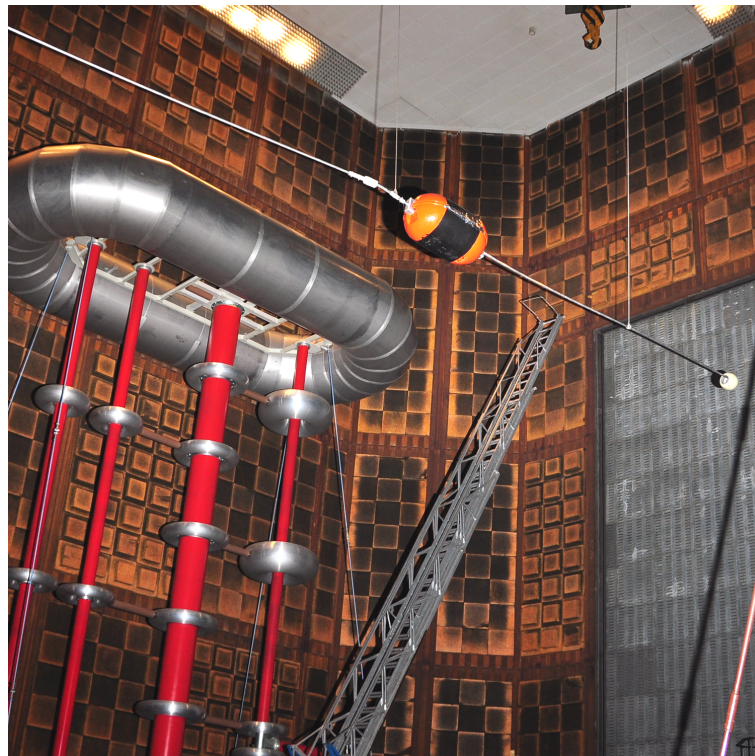
Figure 7.13: Photograph of the setup mounted on a steel pipe during the laboratory high-voltage icing test
