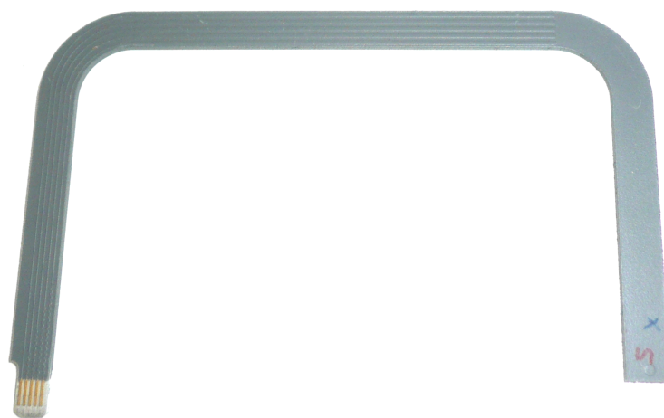
Figure 9.2: Photo of a sensor electrode setup (aluminium based PCB with fluoropolymer coating).
