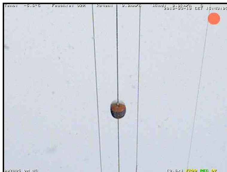
Figure 8.11: Event 1: Weather camera image from March 10, 2010, 3 p.m. [3]. Snow falls and deposits on the test device.
