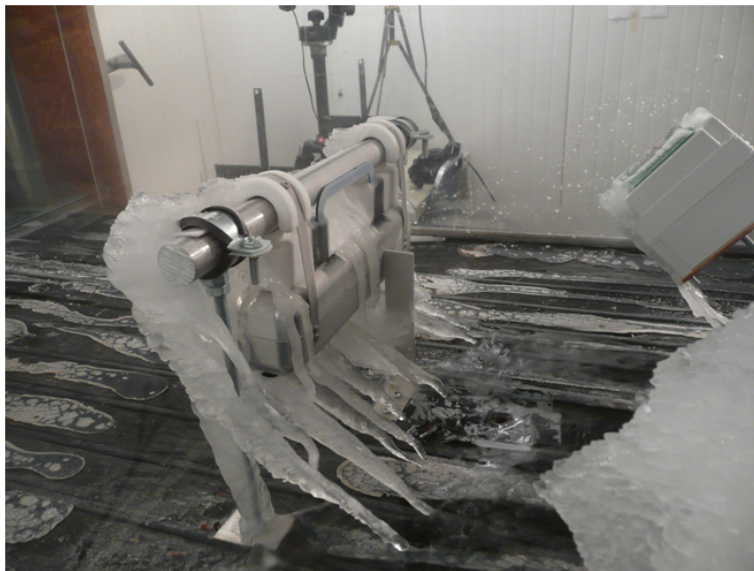
Figure 9.9: Probe in icing tunnel, glaze ice and icicles.
