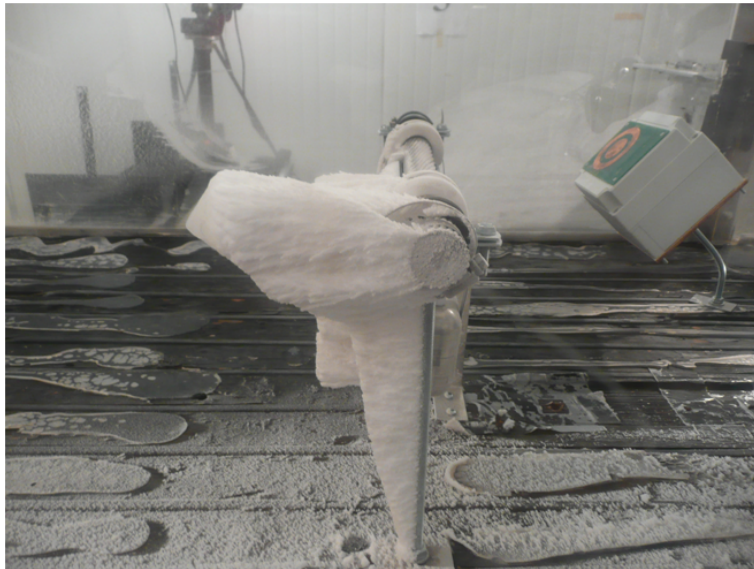
Figure 9.11: Probe in icing tunnel, thick soft rime.
