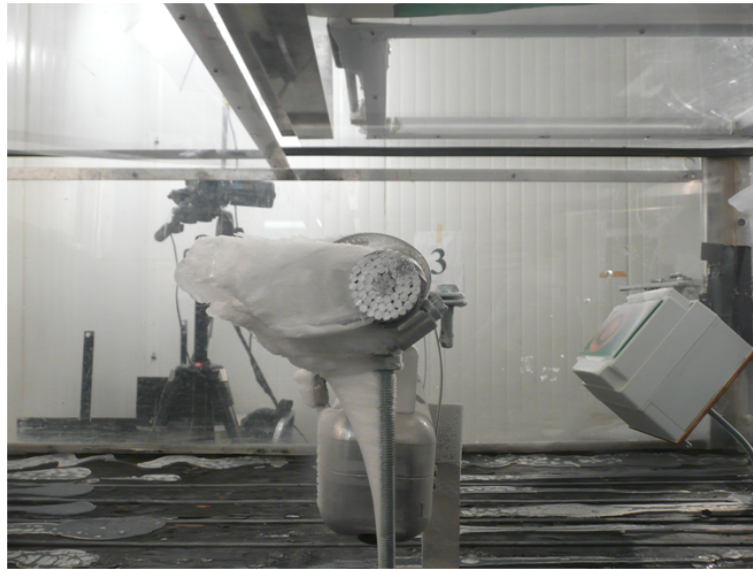
Figure 9.13: Probe in icing tunnel, thick hard rime.
