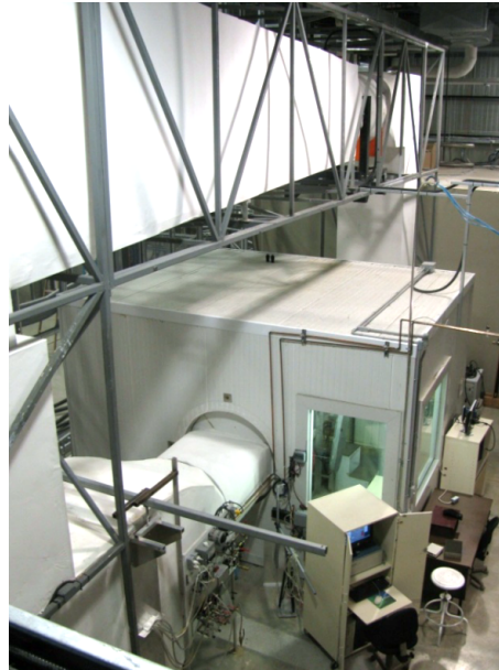
Figure 9.7: Overview of CIGELE Atmospheric Icing Research Wind Tunnel [10].
