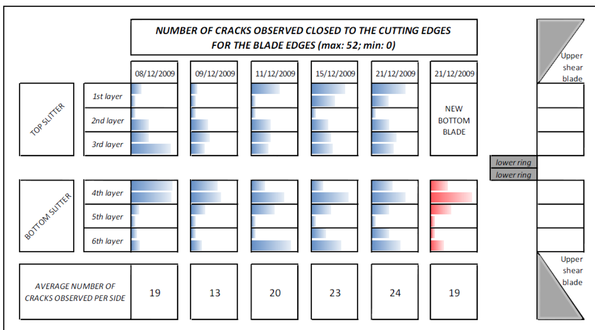
Figure 107: Number of cracks depending on location of sheet within stack as a function of the blade wears (on the blade side)
