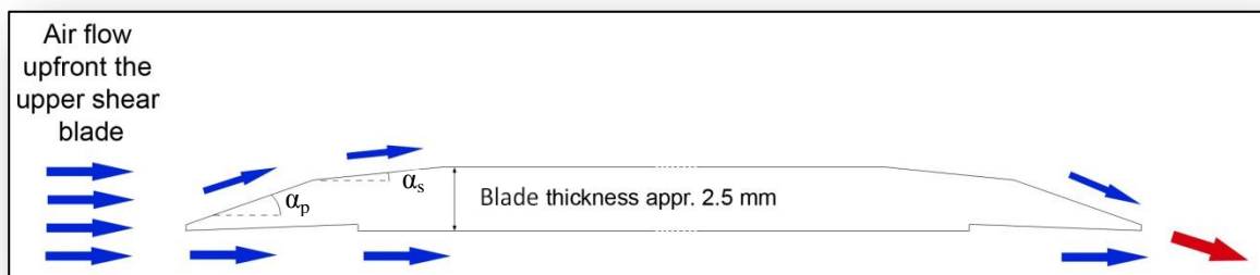
Figure 24: Air flow displacement around the upper shear blade
