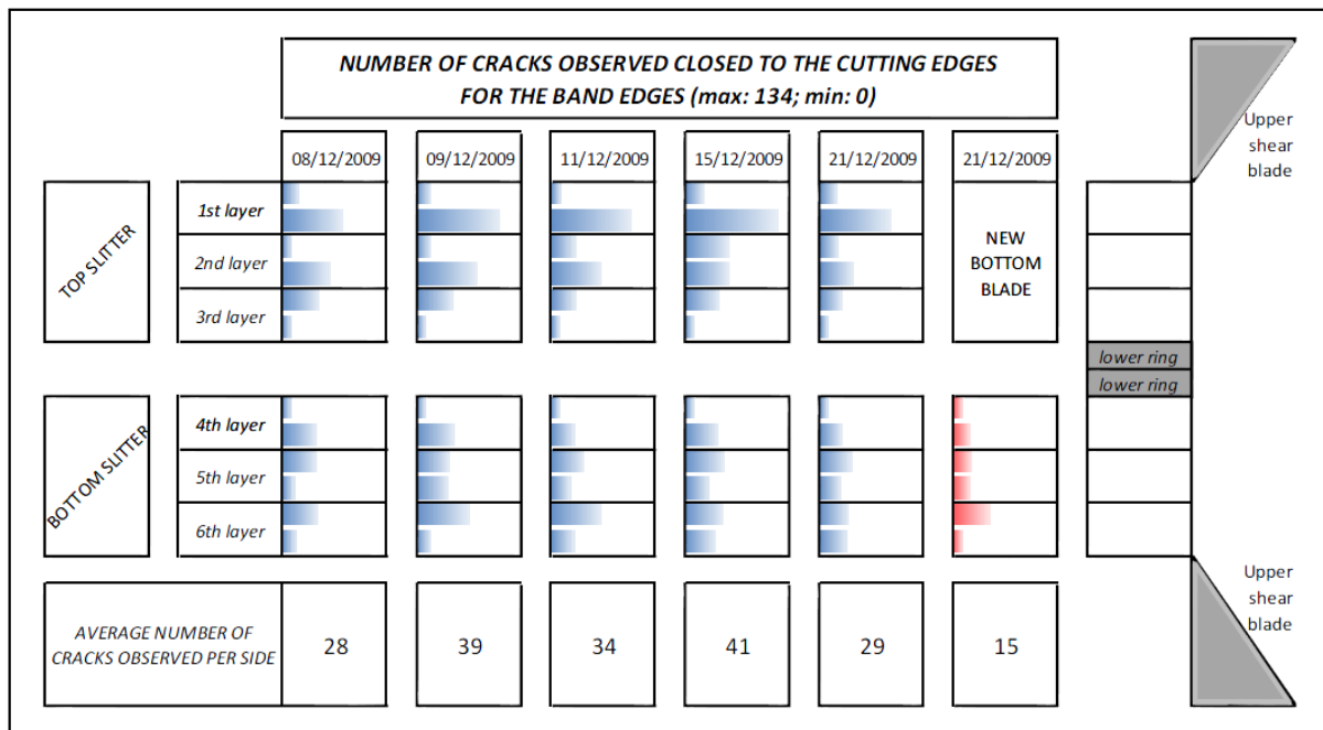
Figure 108: Number of cracks depending on location of sheet within stack as a function of the blade wears (on the band side)
