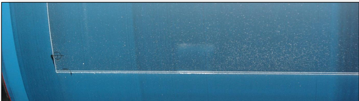
Figure 26: Accumulation of cutting dust on cyan printing blanket (after 5000 cps)
