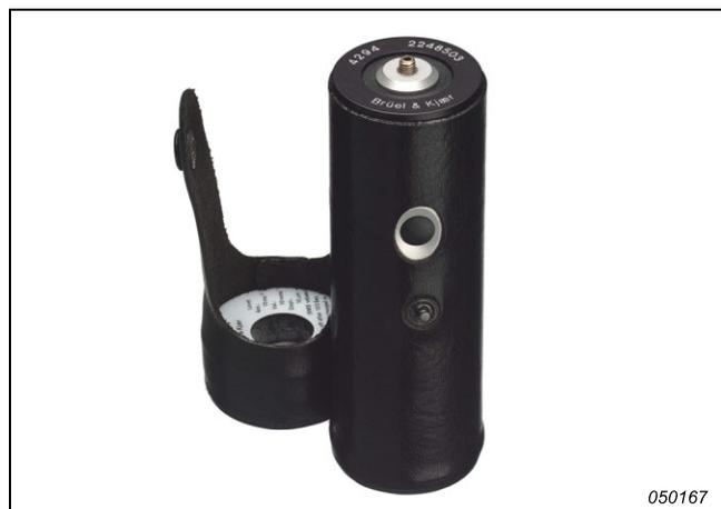
To prevent overload, power for the calibrator is automatically disconnected if a transducer mass above a certain level is mounted on the table (70 g for Type 4294 and 200 g for Type 4294-002).
