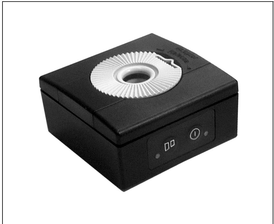
bility and independence of variations in static pressure and temperature around the 1 kHz calibration frequency. The result of this is a user-friendly calibrator where exact fitting of the microphone is non critical and the effects of changes in temperature and static pressure are negligible.
