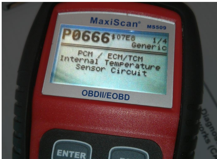
Figure 6-4: Successful DTC readout using the Autel scan tool
