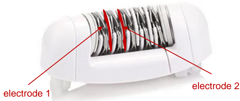
Figure 6-4 Epilation head including electrodes for metal disks
