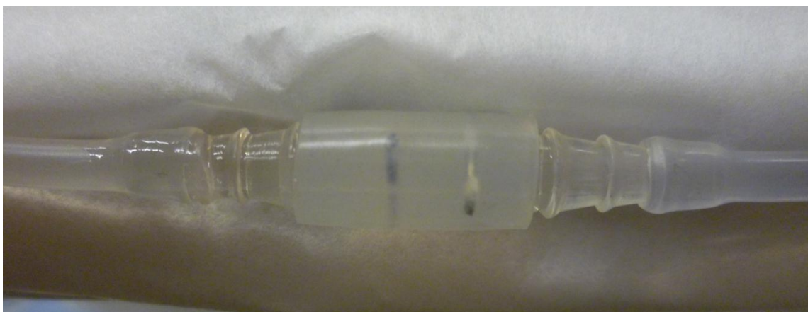
Fig. 3-1 Photograph of a “CROSSER”. Around the “CROSSER” a silicon tube is placed to seal the fitting. Left and right tubes are connected.
