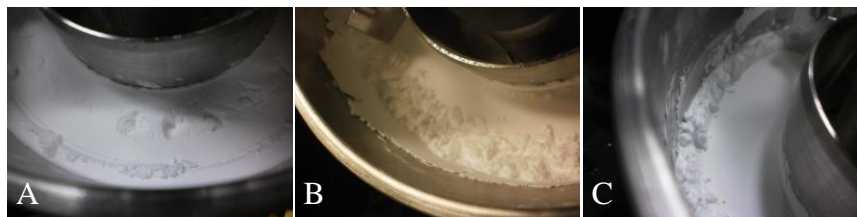
Figure 2-10: Layer conditions: A-Holes in layer; B-Excess powder on the layer; C-Uniform, even powder layer.
