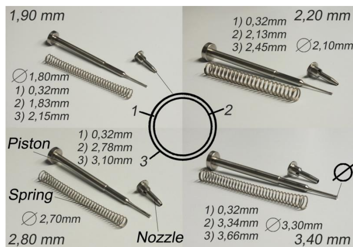
Figure 4-1: Schematic presentation of the low dose dosators
