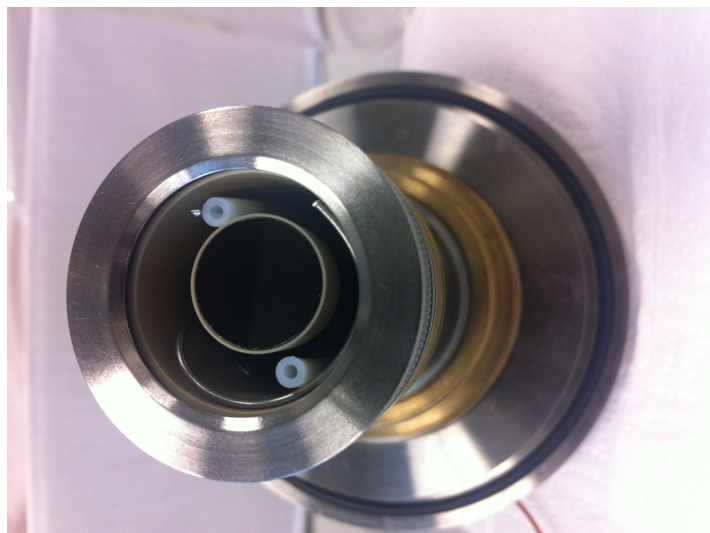
Figure 2.3. Picture of the lower end of the spectroelectrochemical cell showing the in- and out-let tubes, the glassy carbon working electrode and zinc wires as counter (around the WE) and reference electrodes.
