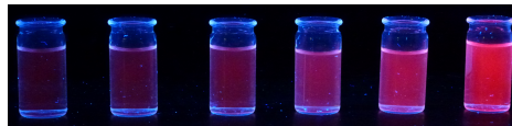
(c) Luminescence of \text{Eu}^{3+} solutions in 50 (left) – 90 v-% acetone in water and in 100 % acetone (right).
