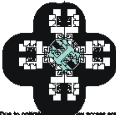
Due to optimizing balcony access areas, one circulation core serves all apartments, communal space erased from floor-level
