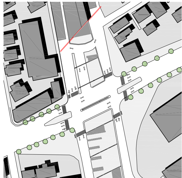
fig. 7 Washington Street: new traffic routing
