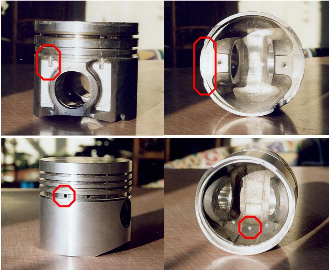
Figure 42: Blow-by gas is guided into the crankcase: around the piston skirt (top)
