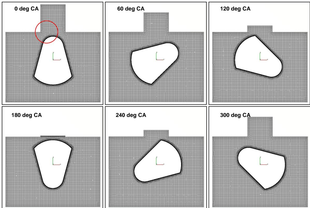
Figure 73: Cuts through the crankweb at 0, 60, 120, 180, 240 and 300 deg CA
