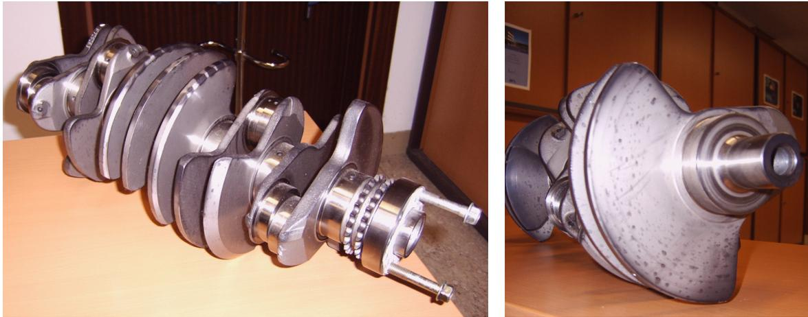
Figure 21: Crankshaft of a V-12 engine
