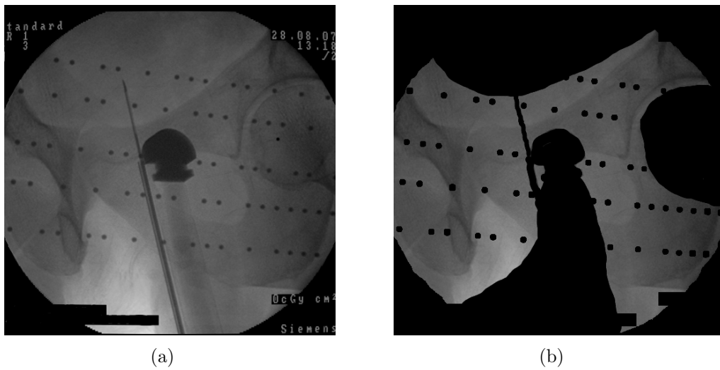
Figure 3.6: The left image shows a radiograph containing different kinds of artifacts such as an ultrasonic probe, a surgical needle, calibration targets, and the camera's aperture. The right image shows the radiograph after the application of w .
