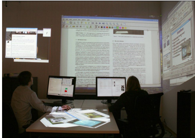
Figure 1.2: Example setup of Deskotheque. The setup contains two standard TFT monitors, three projection wall displays and one table top display, forming a continuous interaction space for two users [Pirchheim2009].
