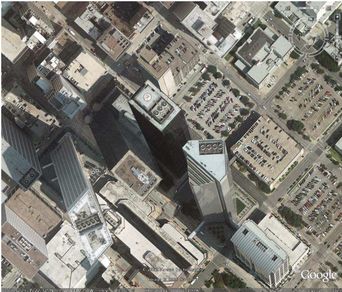
Figure 1.1: View of city center in Houston, Texas as provided in Google Earth. At the border of aerial images the skyscrapers seem to lean into different directions. This is caused by the traditional ortho-image generation method of mapping perspective images onto a 'bald earth' digital elevation model (DEM). Structures that deviate significantly from this DEM, suffer from perspective distortion.
