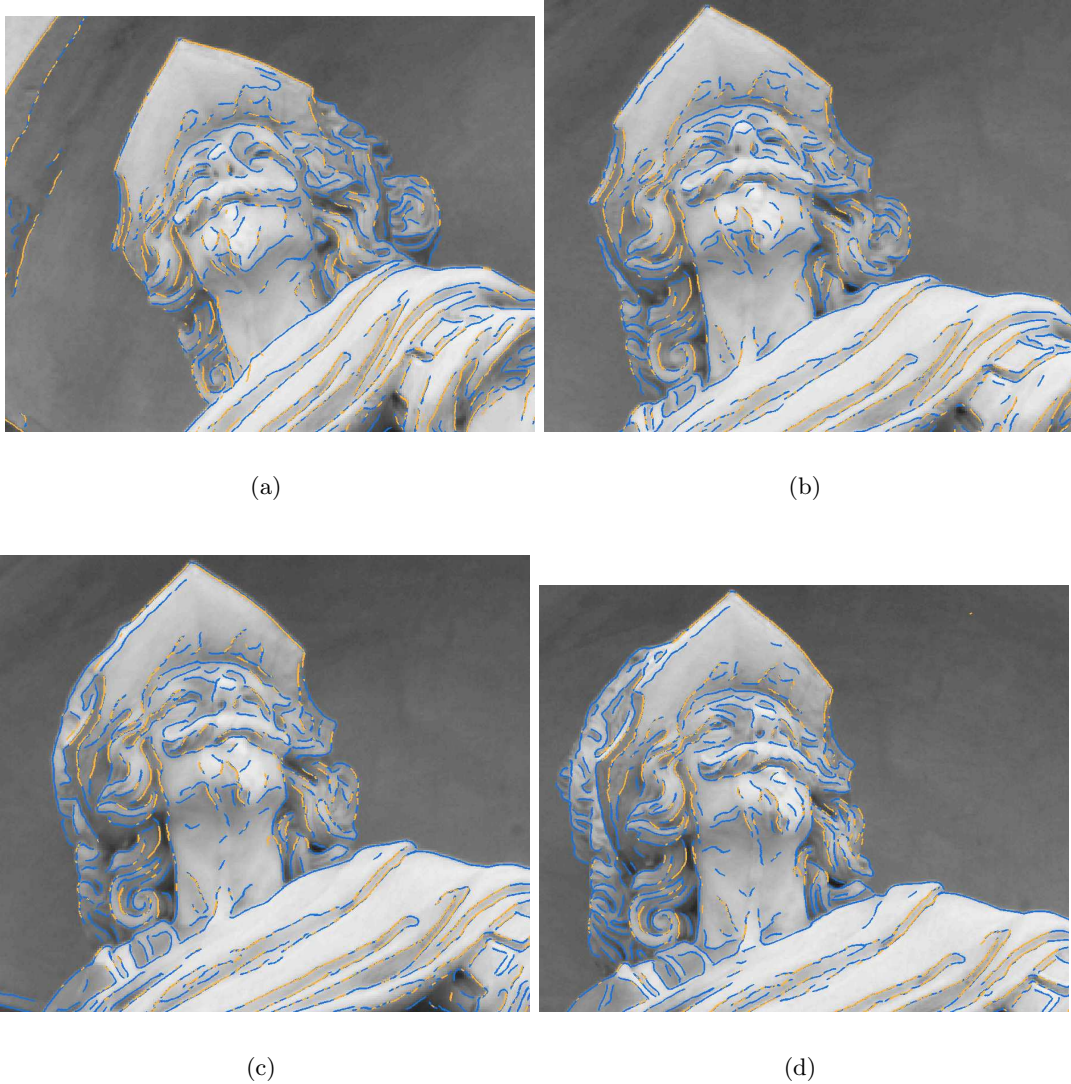
Figure 5.38: Overlays of extracted 2D edgels (in blue) and projected 3D primitives onto four source images. This illustration gives an impression of the reconstruction accuracy by comparing the extracted 2D edgels position to the reprojected primitives position. Furthermore it shows that also for edgels that belong to curved lines a successful reconstruction can be performed. Also notable is the significant change of the images appearance due to large view point changes.
