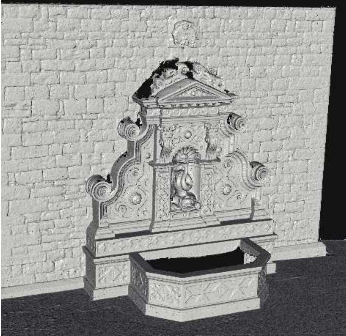
Figure 5.31: Rendering of the triangle mesh of the fountain scene, based on Lidar data. The mesh consists of 12.99 million triangles. The high point density makes this data set well suited for evaluating reconstruction results of image-based 3D modeling methods. The image was taken from http://cvlab.epfl.ch/~strecha/multiview/denseMVS.html
