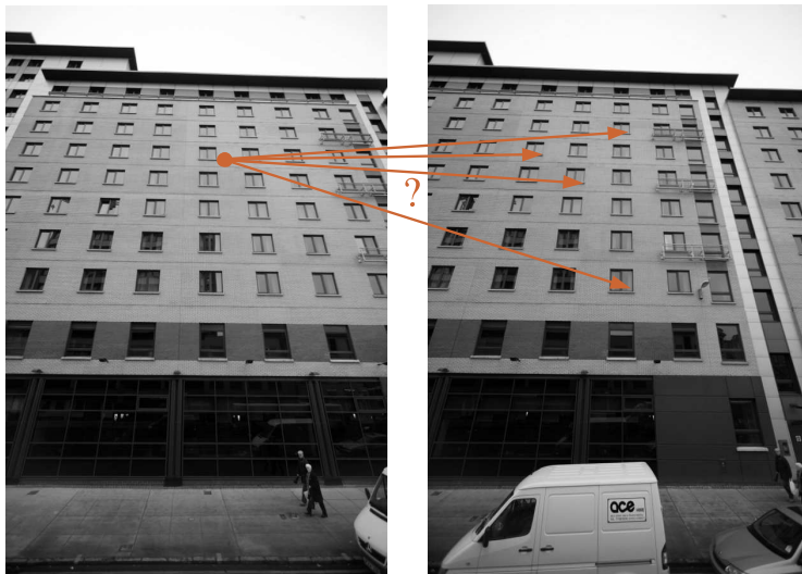
Figure 3.9: Establishing correspondences between views that contain repeating patterns is a challenging task. The window corner marked by the circle in the left image matches with a great number of window corners in the right image.
