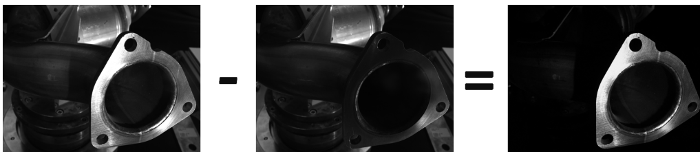
Figure 4.19: Relative intensity measurement. In the presence of stray light, active illumination provides the possibility to subtract the scene with stray light only from the actively illuminated scene [70].
