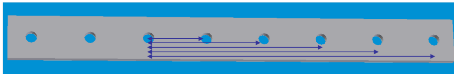
(b) Measured drill holes. The distances between the third hole and rest of the holes to the right were measured with the CMM and with the vision sensor.
