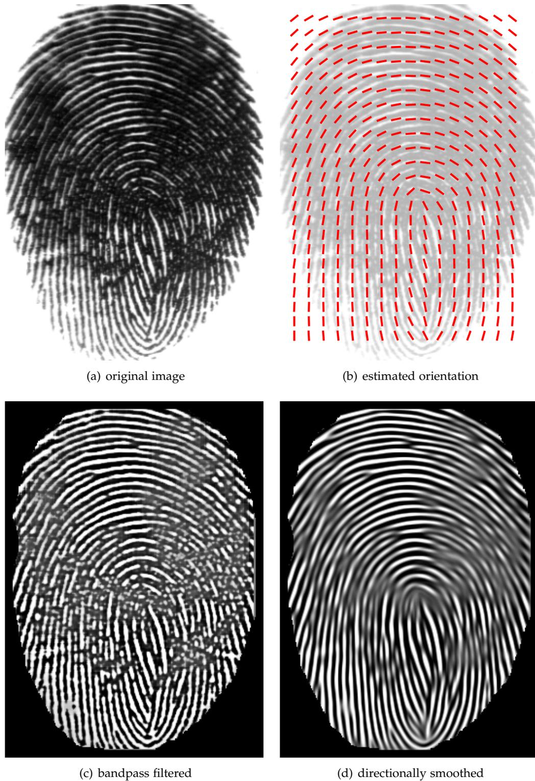
Figure 5.5: **Enhancement example.** The original image (a) is taken from the fvc2004 database 1a and contains ridges which can not be well discriminated from the valleys. The orientation in Subfigure (b) is estimated using the model based procedure as described in chapter 3. The bandpass filtering results in the image (c). The final enhancement including the directional smoothing is shown in (d).
