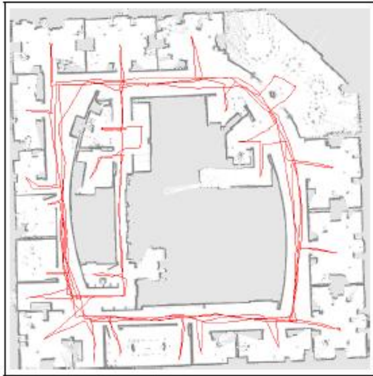
Figure 2.4: High quality indoor map, GridSlam from Hähnel et al. [31] (2003): This indoor map was created with the GridSlam algorithm and 500 particles.
