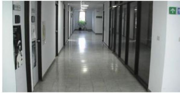
Figure 4.7: Laser range finder problems with window panes, Yang et al. [53]: Laser range finders have problems with mirrors and windows.
