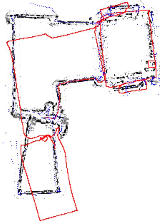
Figure 6.9: Sonar Evaluation on RawSeeds "Bicocca_2009-02-25b" dataset: This map was generated with 12 sonar transducers, a cell size of 20cm and 50 particles. The upper part of the map shows rectangular structures.
