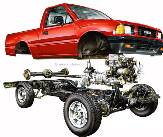
Figure 2.29: Exploded View. The objects have been displaced to resolve occlusions. The presentation uncovers the internals of a car by moving occluding structure out of the line of sight. (Image courtesy of K. Hulsey, www.khulsey.com )
