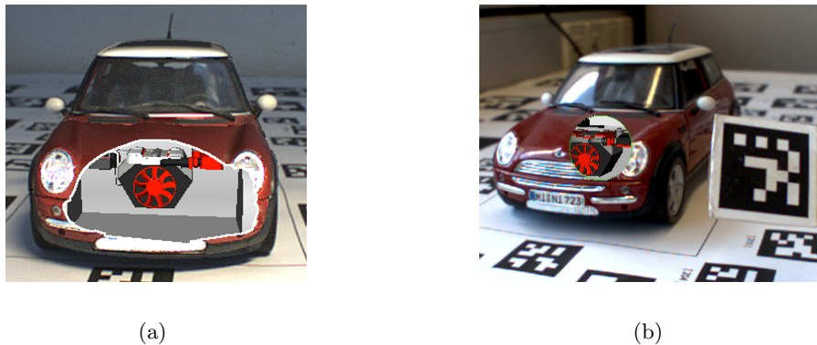
Figure 5.1: Cutaway Presentations (a) Wedge Cut. Notice how the bending of the contour of the cut-out area indicate the shape of the object (b) A Flat Magic Lens controls the cutaway of occluding information. Simple Magic Lens based cutaway classifications are not able to indicate thickness or other occluding structures in-between the occluder and the object of interest. Since no occluding structure is preserved, the presentation fails to indicate the shape of the occluder.
