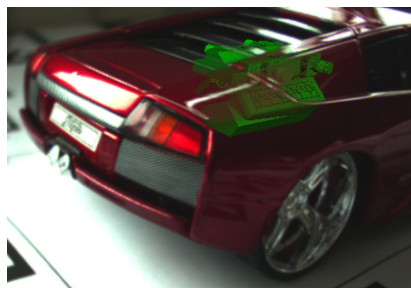
Figure 4.10: Feature Based Transparency Distribution. Edges have been detected in image space and distributed using a 2d distance transform
