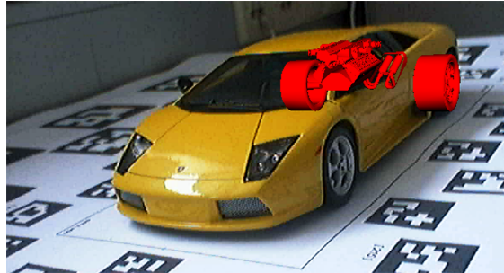
Figure 2.6: A Problem of Depth Perception Even though the virtual objects are correctly registered, they are perceived of as being in front of instead of inside the car.
