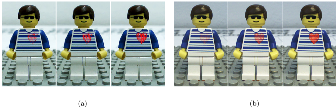
Figure 4.13: Video Ghosting with an Artificial Pattern (a) Video ghosting using a hatch pattern to preserve occluding structure. The pattern is not communicated. Both, hidden objects and occluding texture are difficult to understand (b) Stipple pattern cause less artifacts. However, the hidden object seems to fly in front of the occluder
