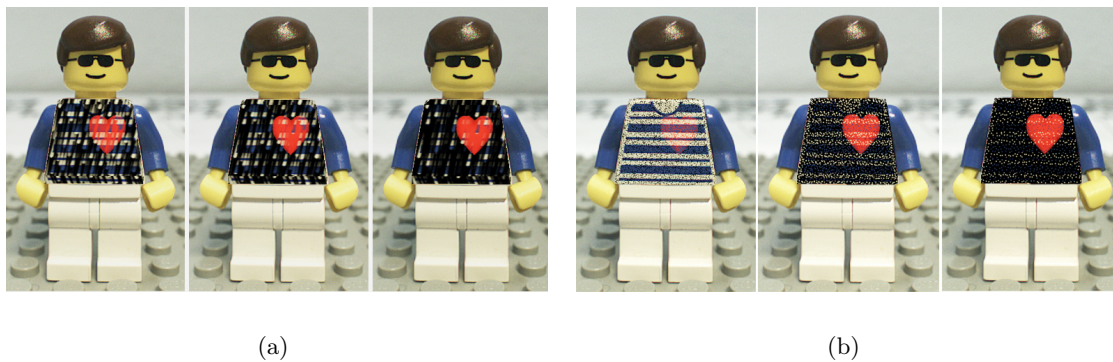
Figure 4.6: Ghosting using Hatching and Stippling in AR on High Frequency Objects (a) Hatching is not aligned with real world texture which results in a disturbed appearance of both (b) Stippling is less interfering with real world texture information if used to control preservation of occluding fragments
