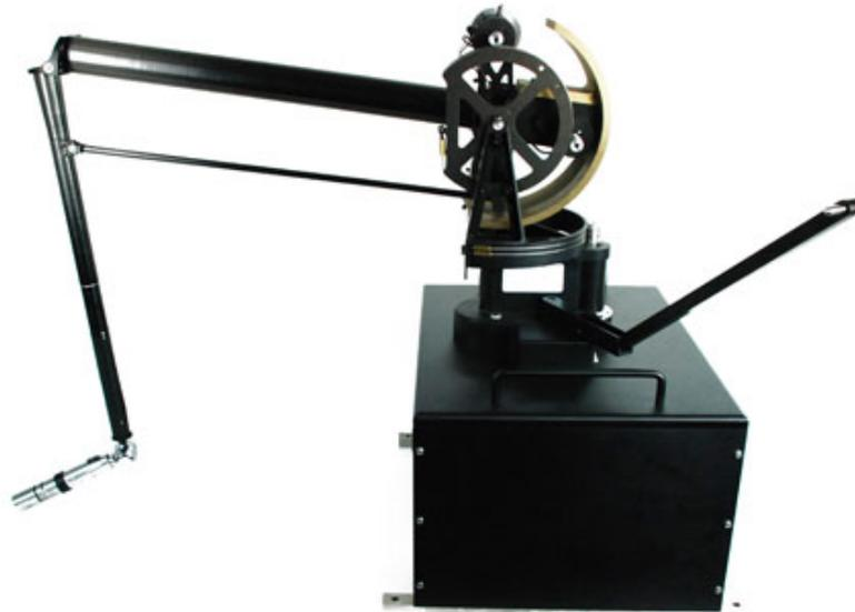
**Figure 8.3:** Force feedback PHANTOM<sup>®</sup> 3.0/6DOF
