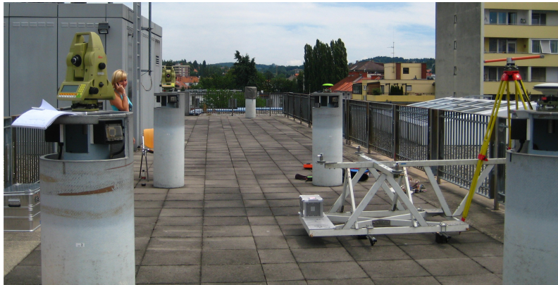
Figure 4.3: Calibration setup of the roof construction by terrestrial measurements
