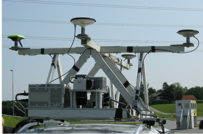
Figure 4.1: Multi antenna array for the attitude measurements
