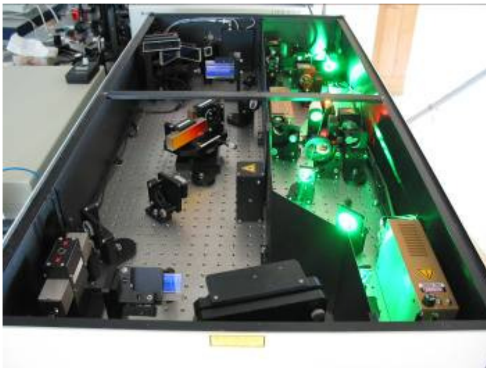
Figure 2: fs-pulsed Ti:sapphire laser at the institute of Nanostructured Materials and Photonics, Joanneum Research GmbH (Weiz, A)
