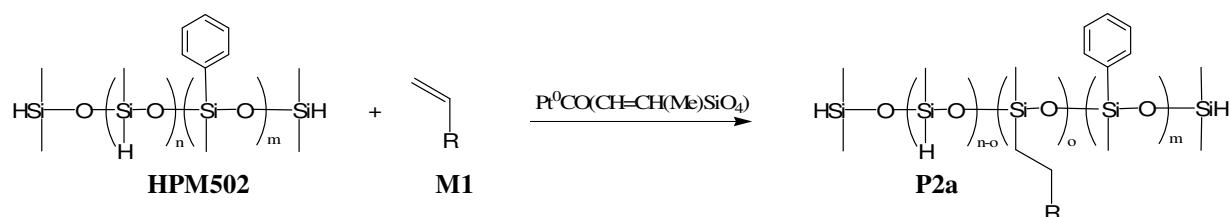
Figure 17: Pt catalyzed hydrosilylation reaction to obtain polymer P3a ; R= 4-(diphenylamino)phenyl benzoate
