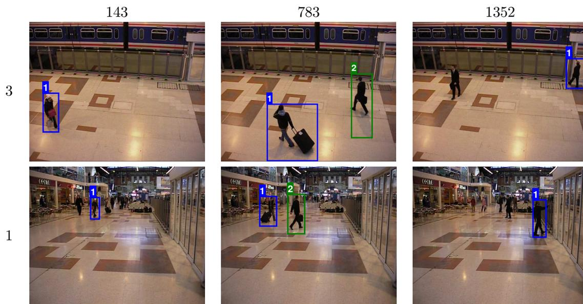
Figure 4.28: People matching between Camera 3 and Camera 1 of the PETS 2006 dataset. The correct match of Frame 1352 is hard to realize only with image features, because of similar intensities. Further difficulties are the low resolution and the wide baseline.
