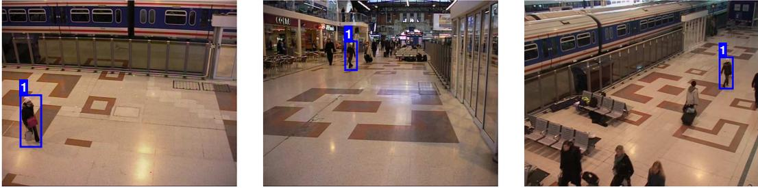
Figure 1.1: Three simultaneously taken images of the PETS 2006 dataset; Camera 3 (left), Camera 1 (middle) and Camera 4 (right). The same imaged person is framed in blue. Note the huge change in appearance which makes visual correspondence so hard. The correct match shows that once the geometry is known, the correspondence problem is simple to solve.
