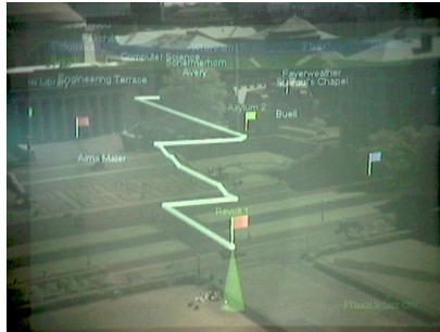
(c) Two examples of augmented scenes captured through the see-through head mounted display. Informations like names of buildings and paths between them can be displayed in 3D, registered with the real world.
