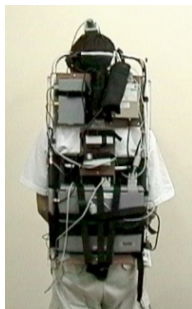
Figure 2.3: Evolution of the Tinmith mobile AR backpack system [40]
