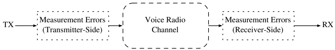
Figure 9.2.: Separation between voice radio channel model and measurement errors.
