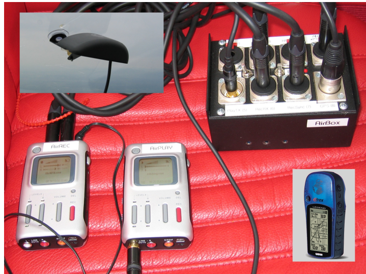
Figure 8.3.: Complete voice channel measurement system on-board an aircraft, with audio player and recorder, interface box, synchronization GPS (top left), and tracking GPS (bottom right).
