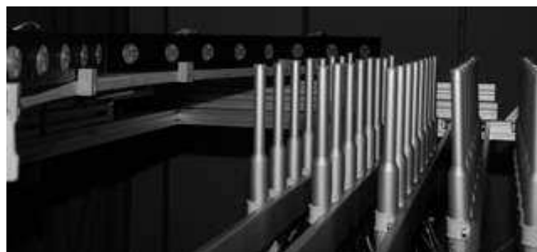
(b) Loudspeaker array with measurement microphones.
