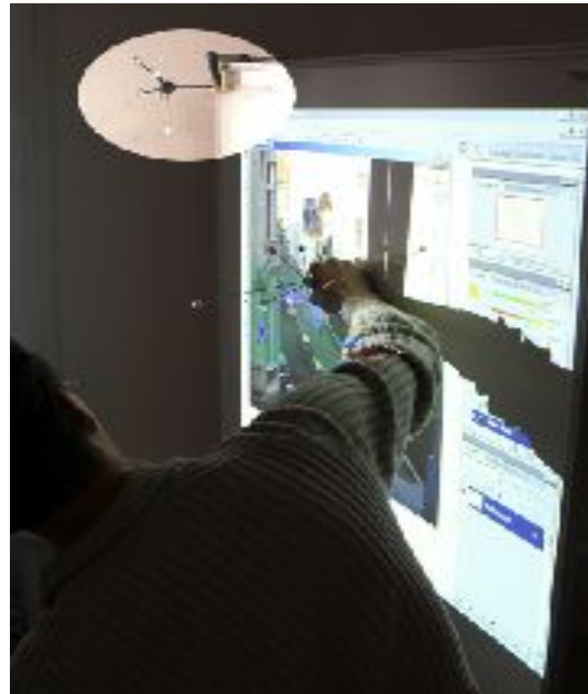
Figure 21: Sketching with Optically Tracked Stylus
