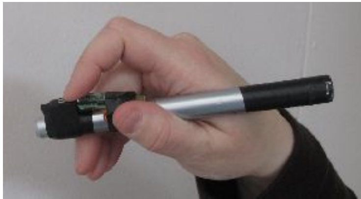
Figure 25: Final Laser Pointer Stylus Prototype
