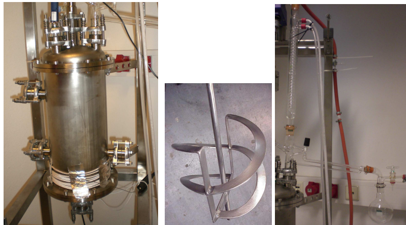
Figure 3-1. (a) Reactor, (b) stirring device and (c) vapour condensation section
