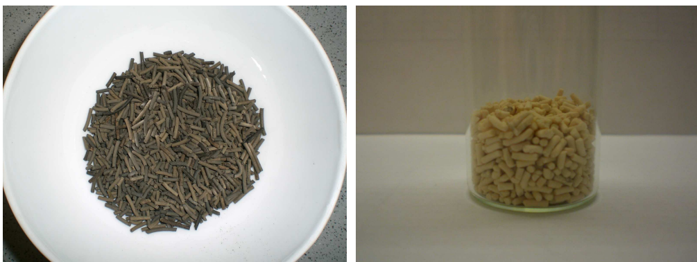
Figure 8-5. Sample photos of the catalyst (a) before and (b) after regeneration
