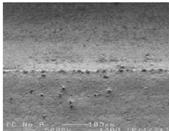
Figure 28 SEM of the PtY-2 catalyst on a microstructured stainless steel foil.
