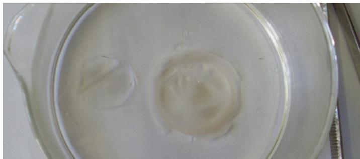
*Fig 5-20: picture of the crosslinked swollen polynorbornene tert-aminobutylester sample in dichloromethane (right) and the empty left glass substrate of the uncured sample*
