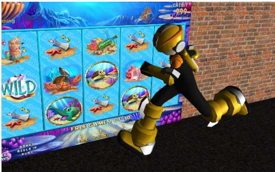
Figure 8.5: An example illustrating the possibility of integrating the 2D surface as a texture object on 3D geometry.
