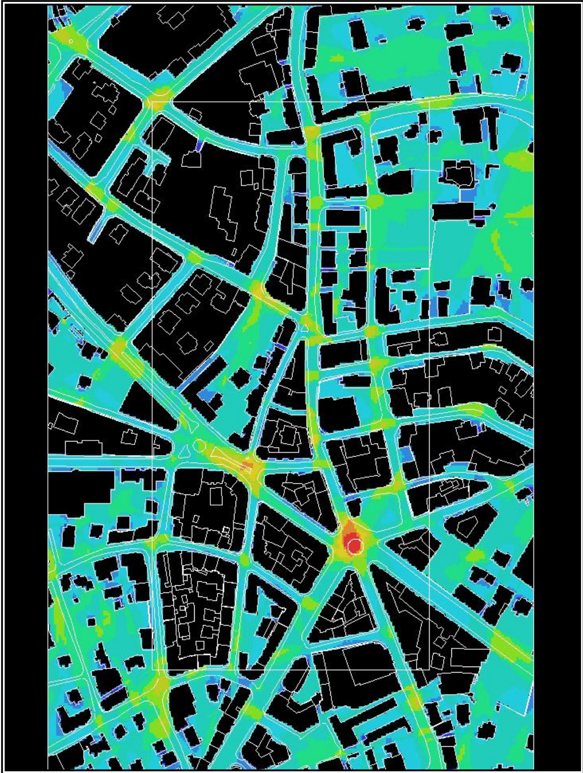
Figure 5-3: Ramallah City Center Control Graph Analysis
