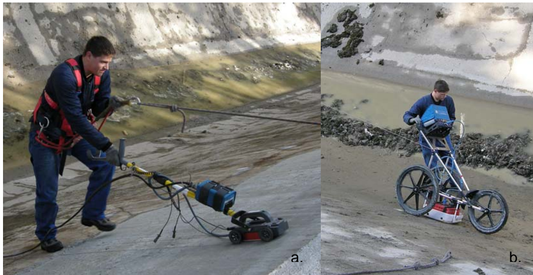
Figure 16. Antennae for georadar surveys
