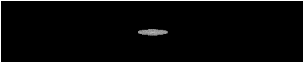
(c) Lowpass-filtering, all frequencies above a cutoff-frequency are set to zero.
