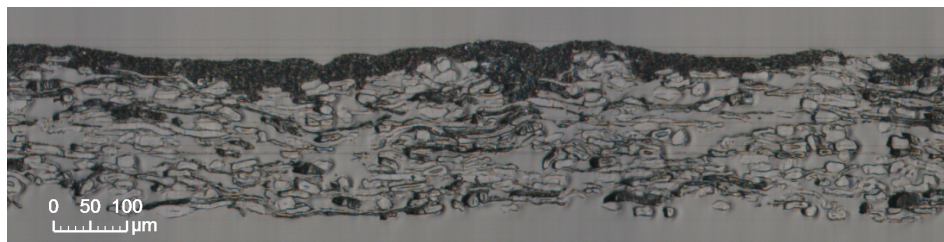
(c) S1Z - Only carbonate containing coating color, low base paper porosity.
