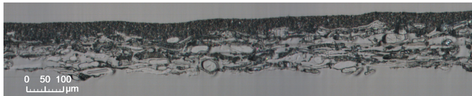
(c) S3S - Coating color 3, industrially produced base paper.
