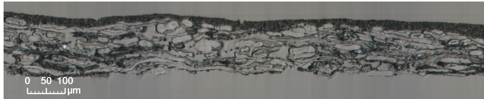
(b) S2S - Coating color 2, industrially produced base paper.
