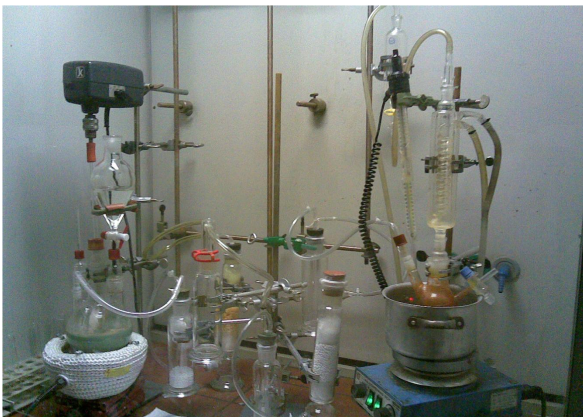
Figure 4-1: Setup for the synthesis of TCPPD using PPD and cyanogen gas.
