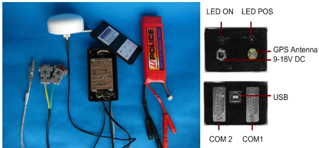
Figure 39: Differential GPS tracking module. (left) A Novatel OEMV-1 receiver (DGPS/RTK) (11x6x3cm) is placed in the middle of connectors, antenna and battery. (right) Side view of the receiver.
