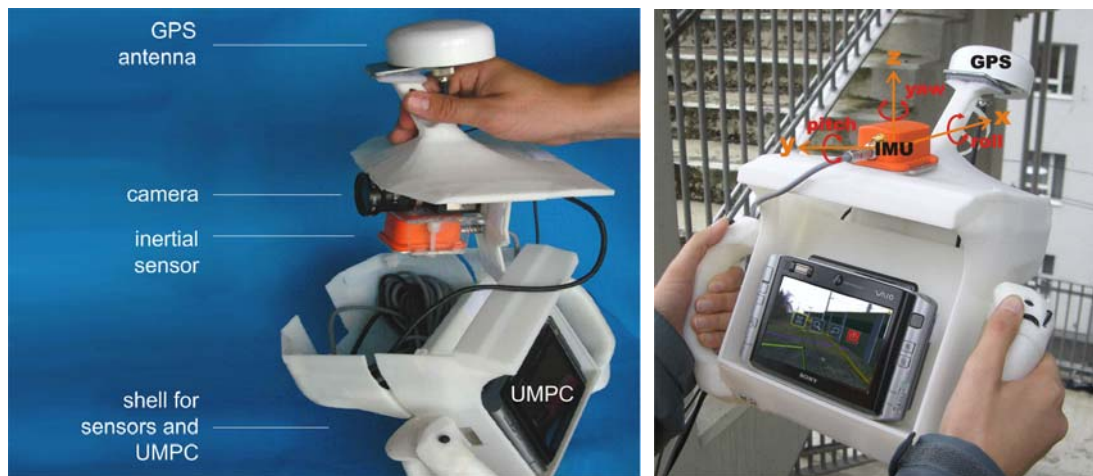
Figure 38: Pomar-3D, outdoor AR setup. (left) Components are protected by a more robust shell. (right) Pomar-3D, outdoor AR setup. User holding the setup for visualization purposes.
