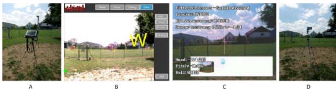
Figure 64: Test setup. (A) Physical mounting and (B) screenshot of the tablet PC-based and (C-D) of the phone-based setups used for accuracy measurements.
