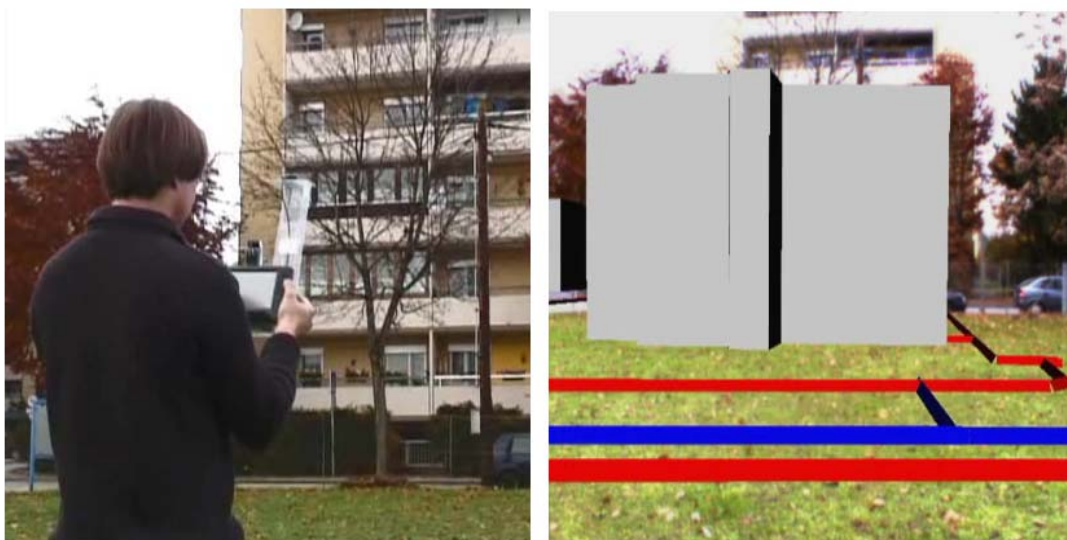
Figure 71: AR visualization of GIS data. (left) User with mobile AR system. (right) Users view of very simple visualization of geospatial data.
