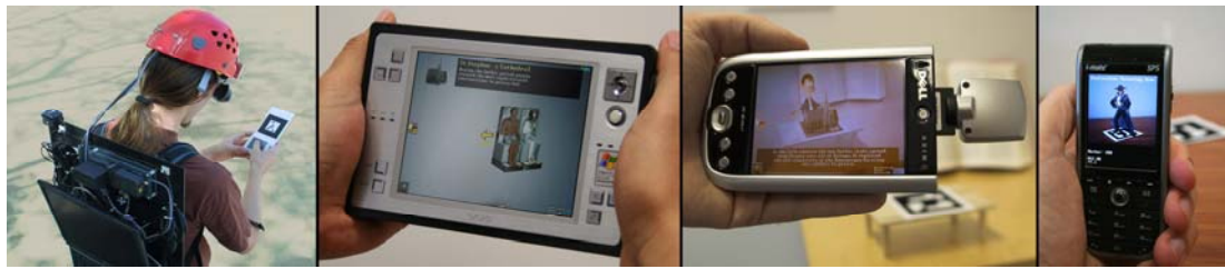
Figure 4: Evolution of mobile AR systems. Hardware setups range from backpack systems to handheld computers.
