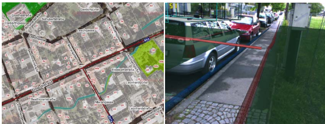
Figure 81: Conventional exocentric view at land register and underground services data as available in two-dimensional GIS visualizations (Graz Geodatenserver) (left). (right) Egocentric view at land register (dark grey on the right highlighting extents of adjacent parcel) and underground services data using AR techniques.
