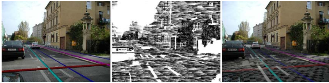
Figure 75: Image-based ghostings. (left) Careless overlay with virtual content, where occlusion cues are not available. Middle: Ghosting map created by this technique. (right) X-Ray view of the same scene using image-based ghostings. The image-based ghosting preserves essential perceptual cues that help to understand the relationship of depth between hidden information and the physical scene.
