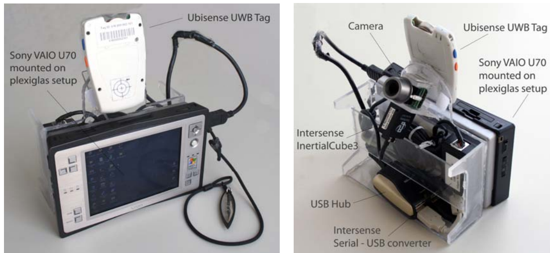
Figure 33: Indoor AR setup. (left) Front view of the mobile device. (right) Back view of the mobile device.
