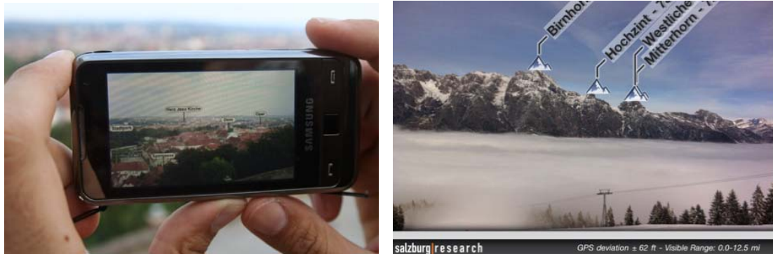
Figure 7: A user operating a smart phone using an AR application for visualizing labels registered on the environment.
