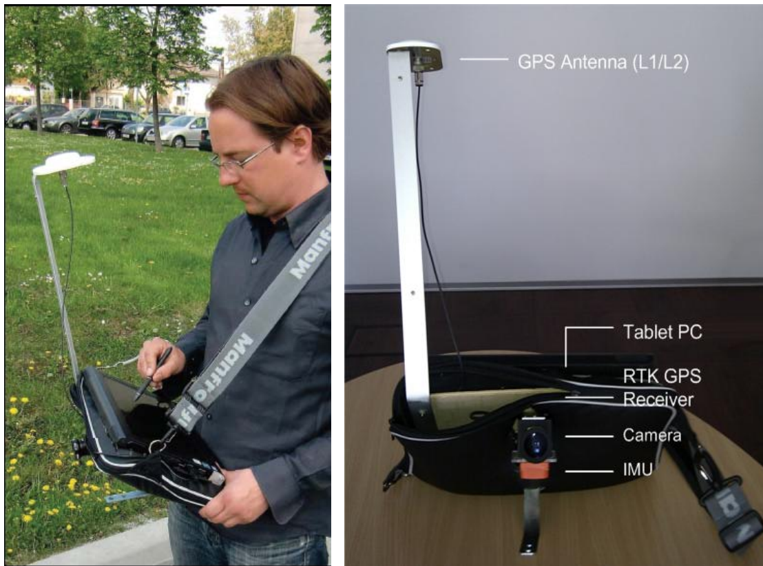
Figure 40: Tablet PC-based AR setup. The user can carry the setup using a carrying belt which allows the AR application to be controlled in a more conventional way.
