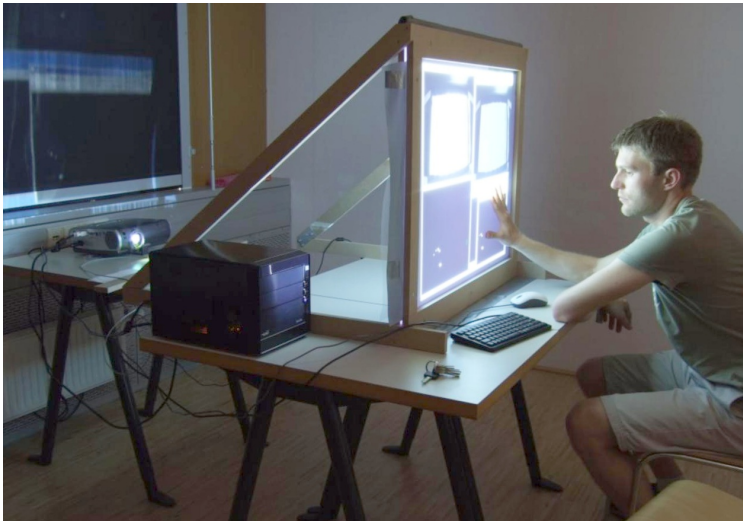
Figure 2.47: An FTIR test setup for the HEyeWall multi touch input. An infrared camera is placed next to the projector to capture the screen. With infrared illumination from the side, the screen lights up when touched.
