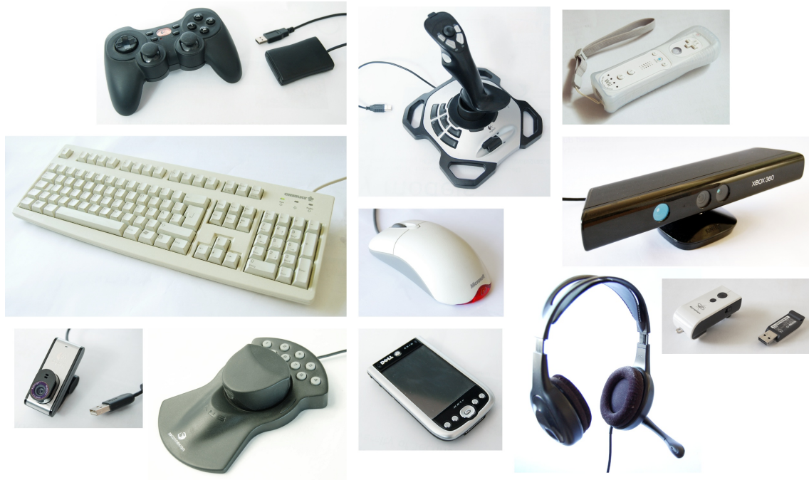
Figure 2.14: A selection of commercially available input devices. Depending on the setup, different devices make sense. Top row (left to right): wireless gamepad, joystick, wiimote. Center row: keyboard, mouse, kinect. Bottom row: webcam, spacemouse, PDA, headset, gyration mouse.
