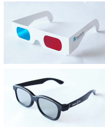
Figure 2.7: Anaglyph and polarized glasses are common technologies to realize cheap stereoscopic displays.
