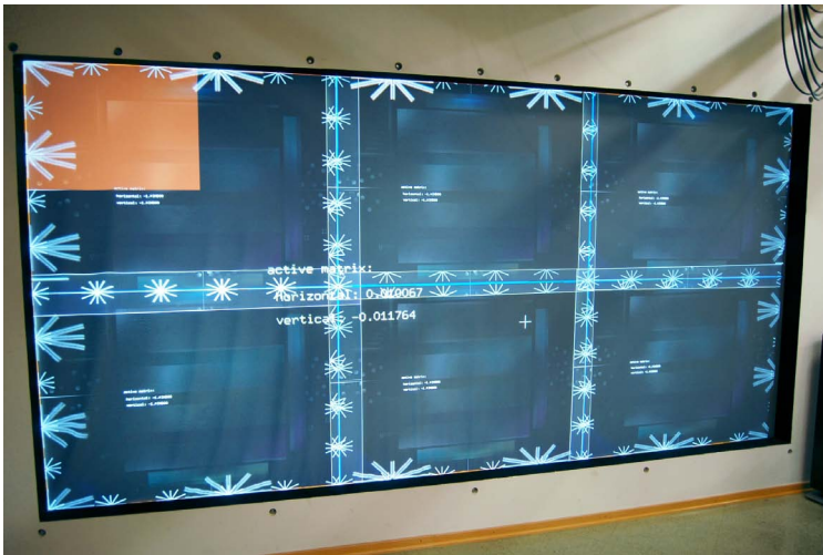
Figure 4.23: Manual geometric calibration of the six high resolution tiled projectors plus one large projector.
