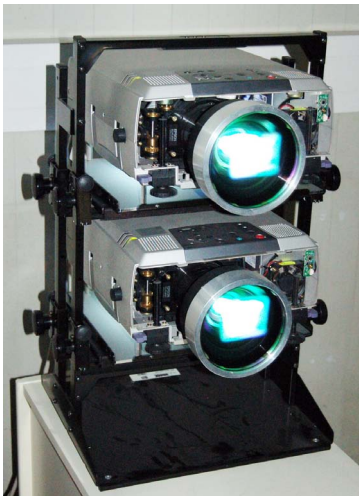
Figure 2.38: A stereo rear-projection setup with two projectors and linear polarization filters attached to the lenses.
