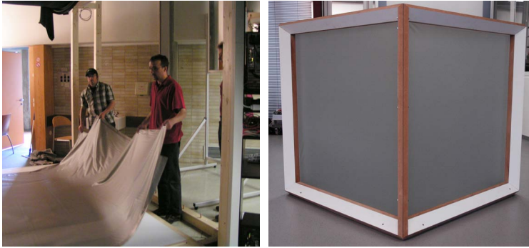
Figure 2.25: Left: With the old frame design, exchanging the screen material is a lot of effort. In this case, the front side was manufactured 1cm too wide and the whole screen had to be exchanged. Right: New frame design by digitalImage. Photo courtesy of Armin Zink.
