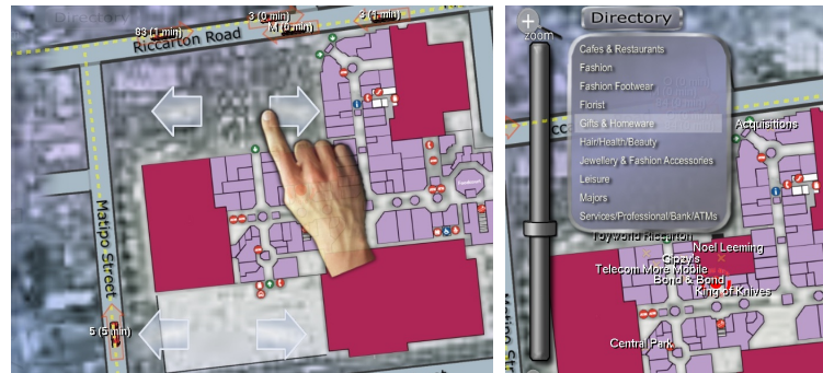
Figure 6.4: Zoomable map with real time bus information. A moving image of a hand illustrates possible interaction and animates passers-by to try themselves (left). Zooming closer, shop names are displayed, also allowing to only show the names of a certain category of shops (right).
