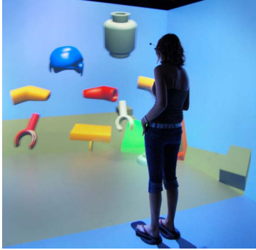
Figure 5.5: Picking and moving objects. Picking is started by ray intersection on a joystick button press. Relative motion and rotation of the joystick are then applied to the object.
