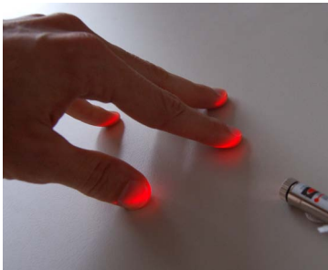
Figure 3.26: Laser Light Plane setup. Fingers entering the plane light up. As they shadow fingers behind, multiple laser line modules can be placed around the screen. Here, a normal table surface turns into a multi touch surface with cheap components.
