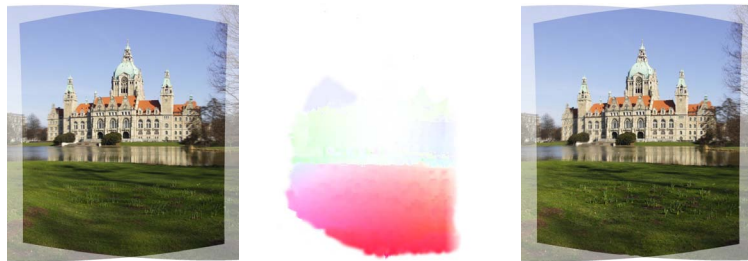
Figure 6.12: Panoramic stitching with a slight camera motion. Without correction, ghosting artifacts appear in the grass area (left image). The optical flow is computed (center image ) and used to warp one image to eliminate ghosting (right image).
