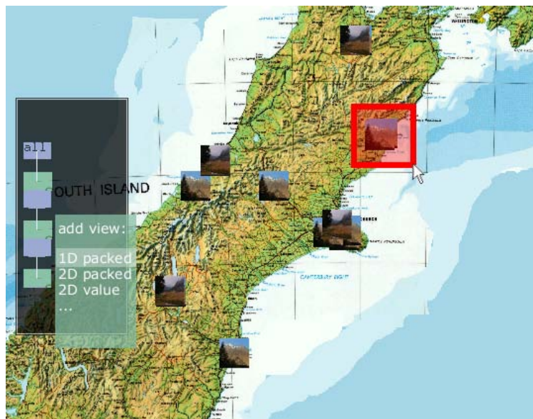
Figure 6.40: Early interface prototype for a fast, zoomable photo browser. To quickly find a photo, the user can subsequently add filters to a filter graph (left) and use a drag (red box) to define the filtered values, e.g. dragging a rectangle on the map to restrict the selection to all geotagged photos within that area.
