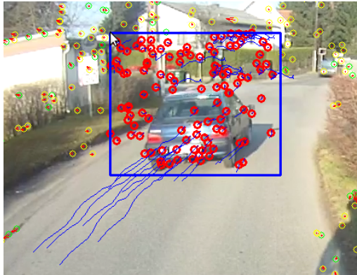
Figure 5.1: Visualization of collected trajectories (blue lines) in a region of interest (blue box)
