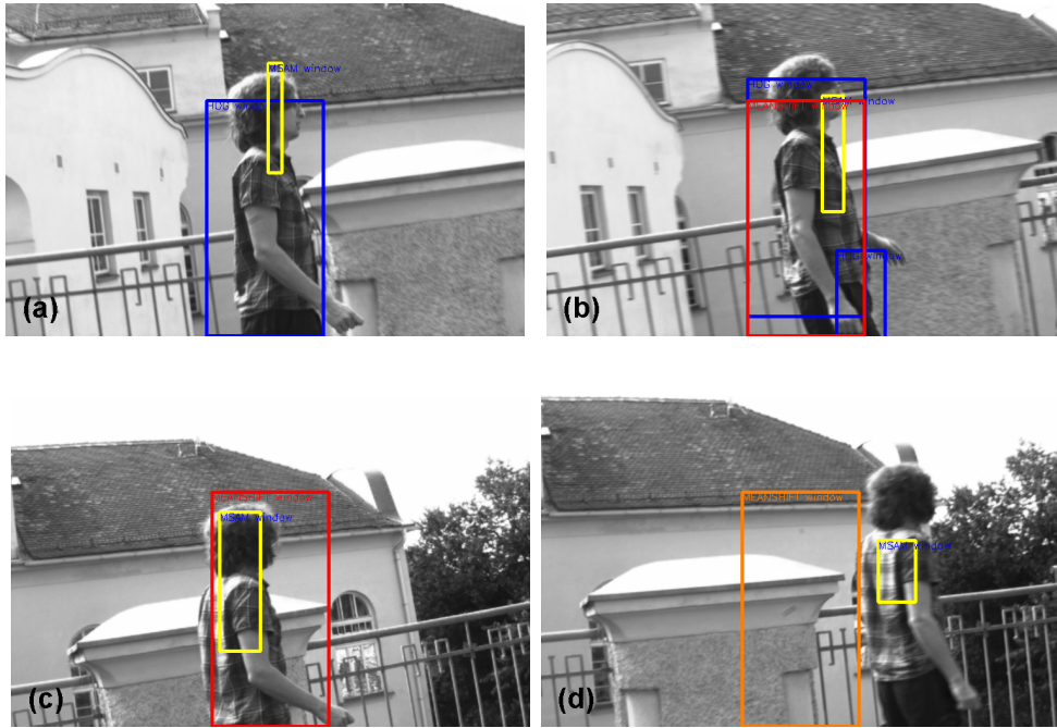
Figure 4.5: Experiment VMG_Person_01: 3D-output back-projected to the image-plane. 3D-output back-projected to the image-plane. Overlap of HOG and MSaM initializes hybrid tracking (red) (a); hybrid tracking (red), MSaM tracking (yellow), and HOG detections (blue) (b); no HOG detection (c); hybrid tracking lost target (orange), deactivation of hybrid tracking is imminent (d).
