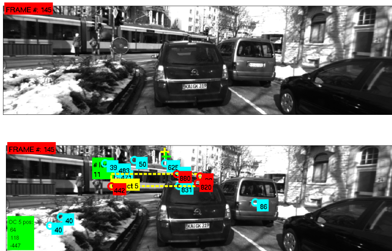
Figure 3.18: Tram detection vs. no tram detection due to a different cluster size in experiment KIT_Seq_04.
