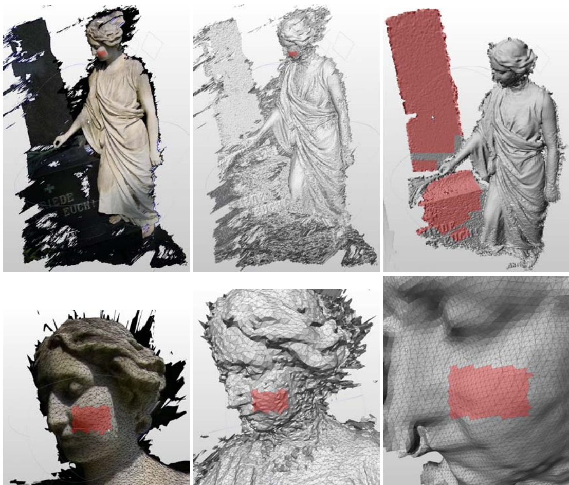
Fig. 5.1 Creating a scanned artifact. Simplified versions of the range maps, textured and un-textured. A rectangular region is marked in different triangulations. Several range maps are integrated and smoothed. The gravestone is manually segmented for a semantic markup.
