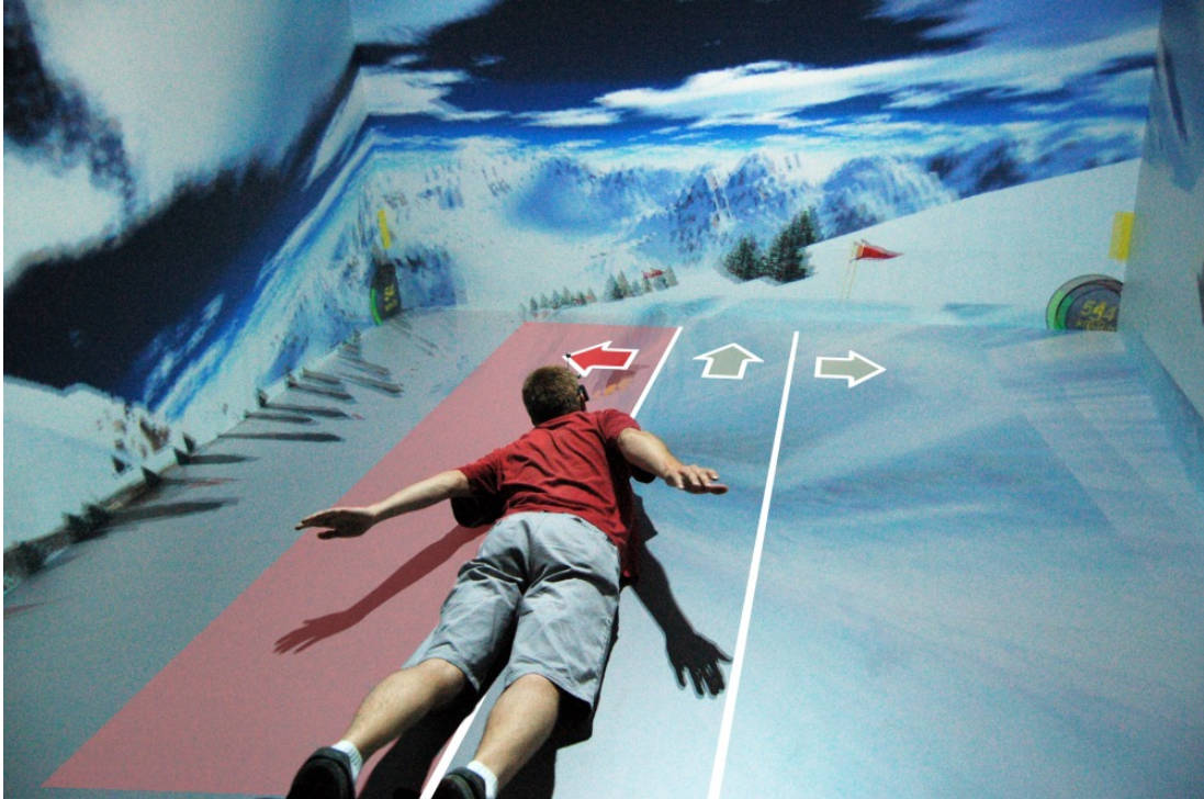
Fig. 4.36 Hands free navigation. A user controlling a penguin by his head position. The arrows and lines are overlaid on top of the photo for illustration purposes.
