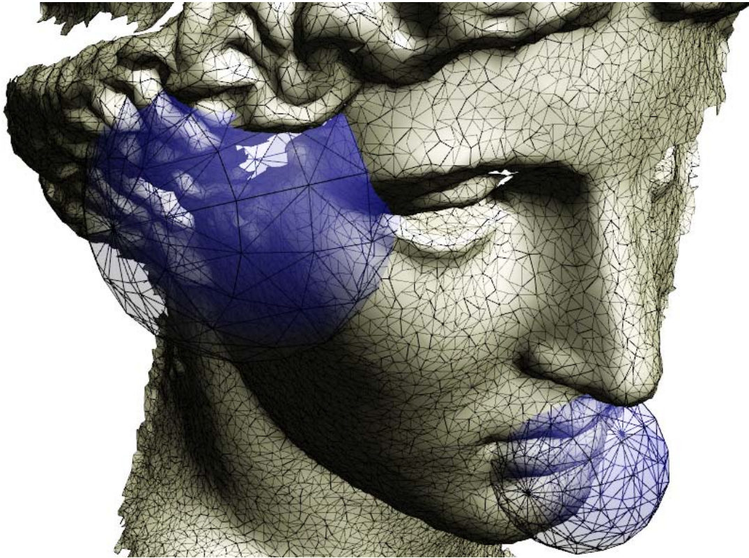
Fig. 3.15 A 3D model file with embedded annotations. Blue spheres have URLs attached.
