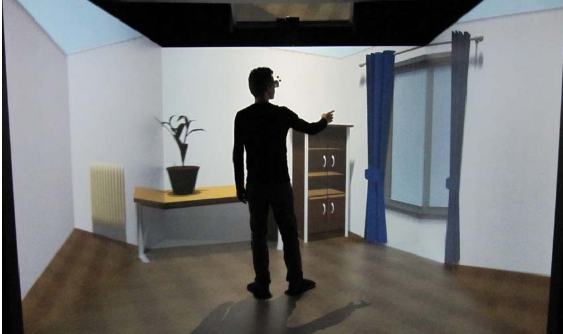
Fig. 4.6 The SweetHome3D output is transferred with our web service to an OpenSG CAVE application which lets the user walk through a 3D representation of the house plan.
