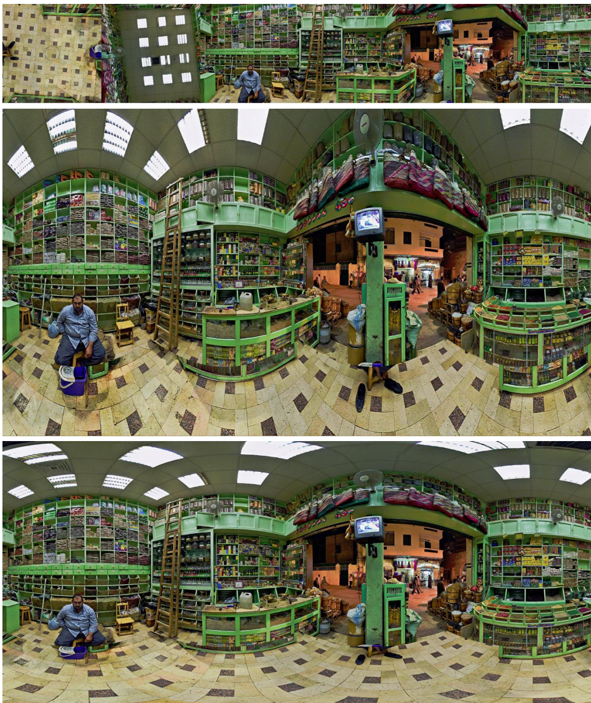
Figure 3.32 Different Formats for Panoramic Images of a Spice Shop in Aswan, Egypt: Cubic Format (Top); Cylindrical Projection (Center); Equirectangular (Spherical) Projection (Bottom); [258]
