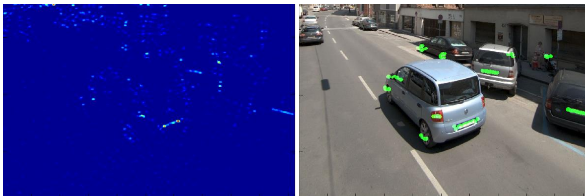
Figure 4.20 Sample Response S from License Plate Filter (Left); Input Image with Resulting Detection Masks from License Plate Detector (Right)
