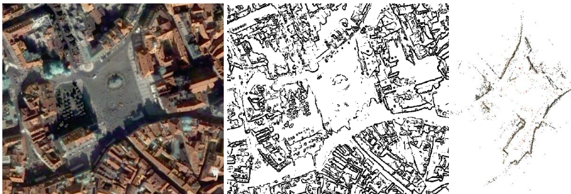
Figure 7.3 Example from Kaminsky et al. [14]: Overhead Ortho-Image of Old Town Square in Prague, Czech Republic (Left); Corresponding Edge Image (Center); Overhead View of Structure-from-Motion Point Cloud Obtained from User Photos using Photosynth (Right);
