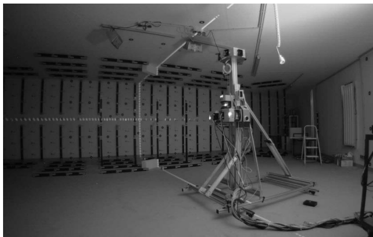
Figure 4.9 Infrared Laser Pattern Used for Determining Exterior Orientation of Laser Scanners
