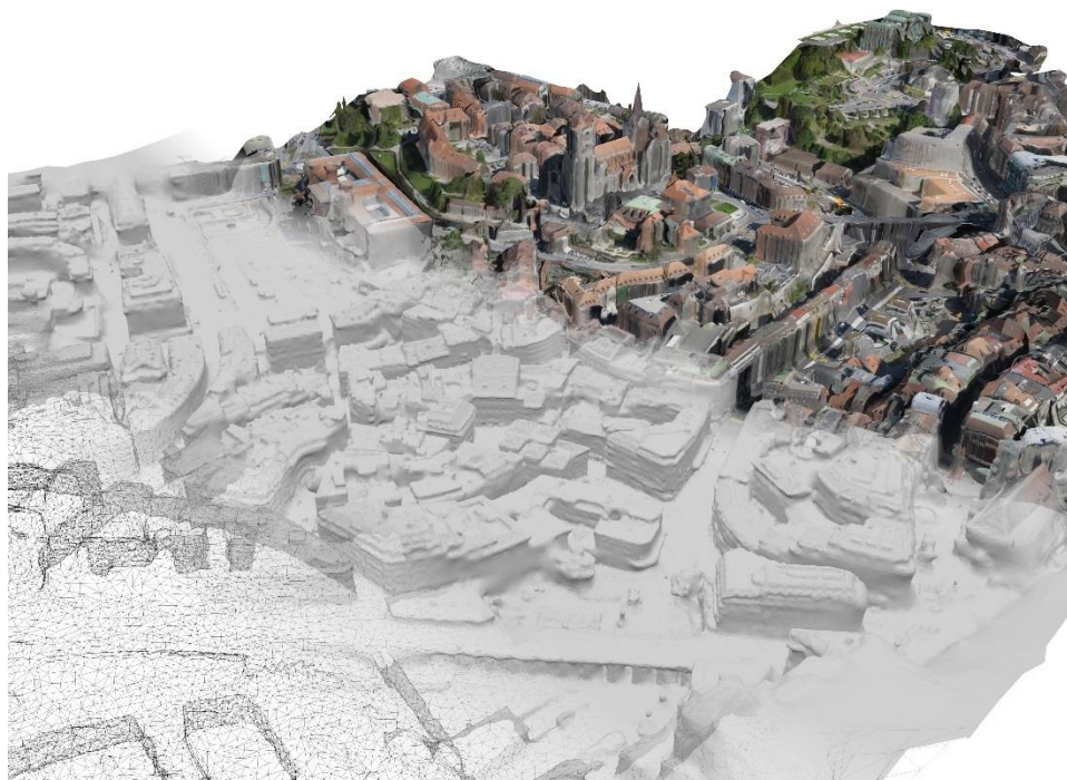
Figure 3.18 Textured Surface Model of Laussane, Switzerland, Generated from UAV Imagery using Pix4D Workflow; [230]
