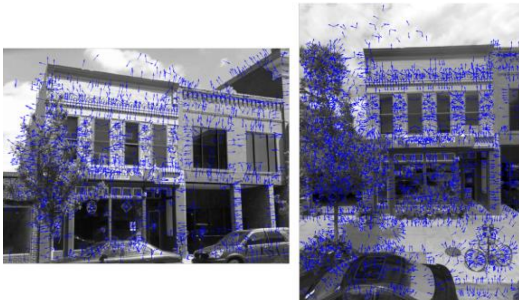
Figure 5.10. Sample pair of query image (Left) and Part of Search Panorama Image (Right) Showing Orientation Vectors of Detected Interest Points.
