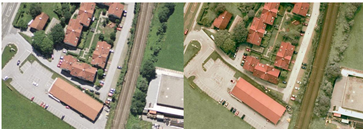
Figure 3.22 Comparison of Film Based Image (Left) and UltraCam-D Image @17 cm GSD (Right)
