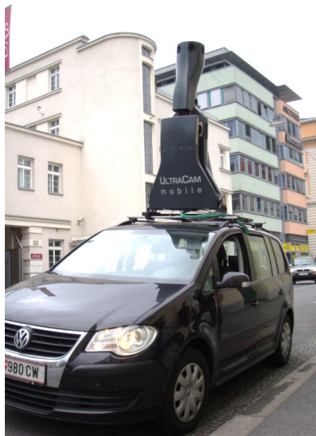
Figure 4.14 UltraCam-M Mobile Mapping System v1 Installed on Capture Vehicle
