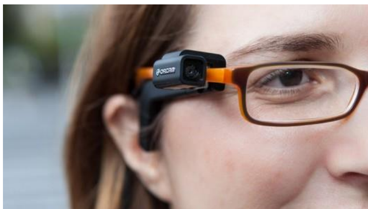
Figure 3.40 "OrCam" Wearable Computer Vision Enabled Device offering Visual Object Recognition for the Visually Impaired [296]
