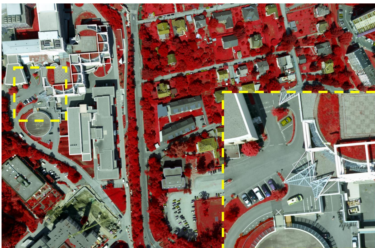
Figure 3.24 Level-3 False Color Infrared Image Captured with UltraCam-D Camera at 4 cm GSD; Red Colors Indicate Vegetation; Location: Children's Hospital in Graz, Austria;
