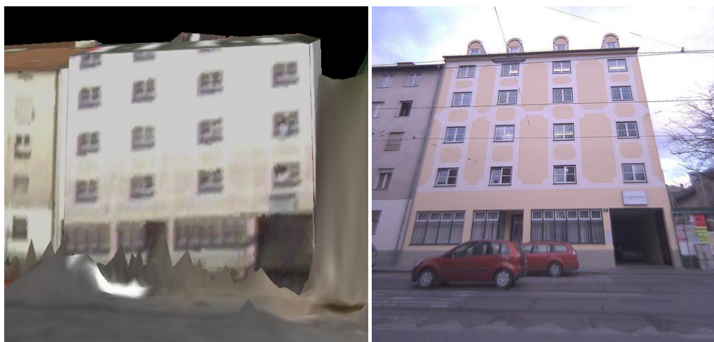
Figure 4.3 3D Building Model Textured with Aerial Imagery at 30 cm GSD (Left) and Potential Improvements using Streetside Image Captured at 2 cm GSD (Right).
