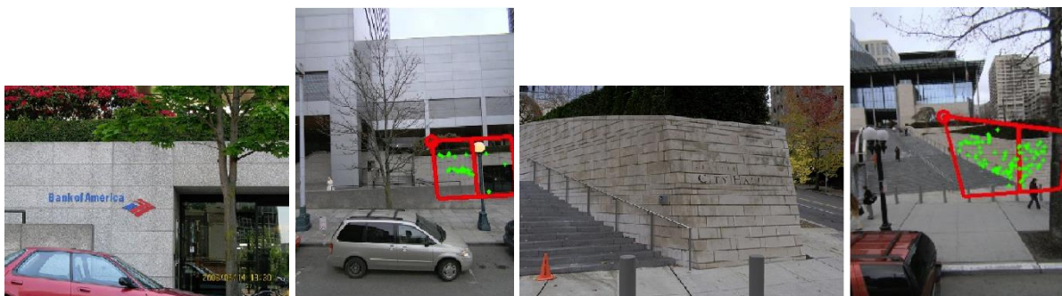
Figure 6.9 Examples of Successful Matches with Minor Overlap between Query and Index Images; Detected Bounding Polygon is Shown in Red, Matched Feature Points in Green;
