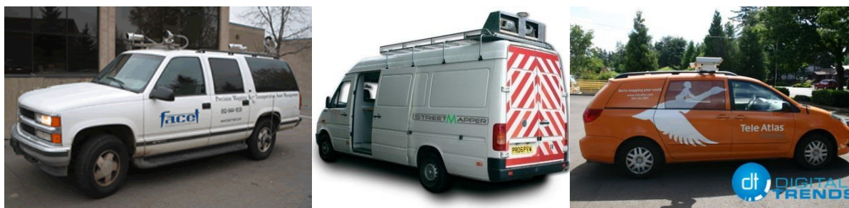
Figure 4.2 Different MMS available in 2005 and 2006: [246] MMS for LBS Data Capture (Left); [248] Street Mapper MMS for Precise 3D Mapping (Center); TeleAtlas MMS for Street Mapping (Right) [312];
