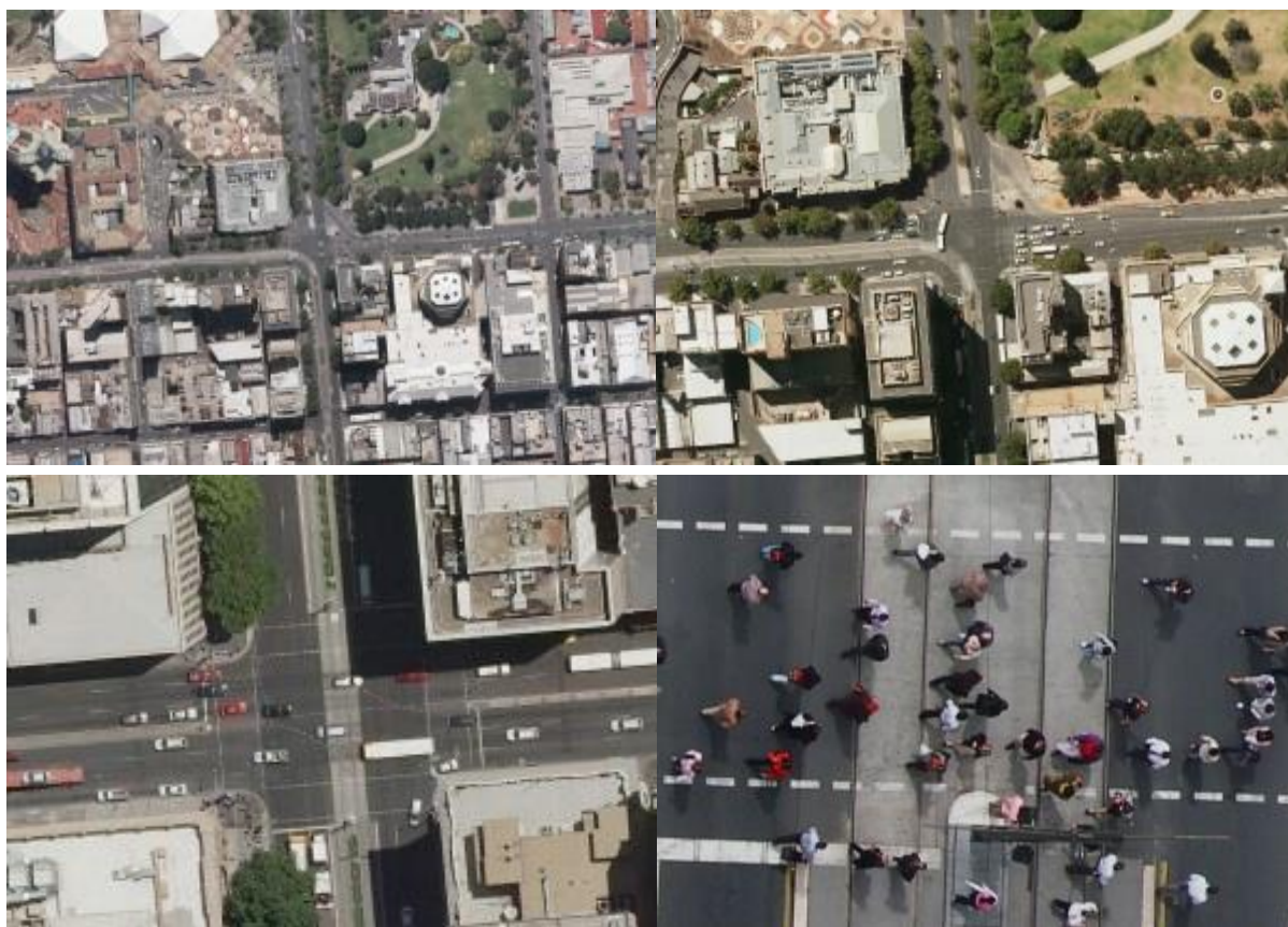
Figure 3.10 Comparison of Satellite and Aerial Imagery of the Same Location: IKONOS Image @ 1 m GSD (Top Left); WorldView-2 Image @ 0.5 m GSD (Top Right); UltraCam-D Image @ 20 cm GSD (Bottom Left); UltraCam-X Image @ 2.5 cm GSD (Bottom Right); [198]
