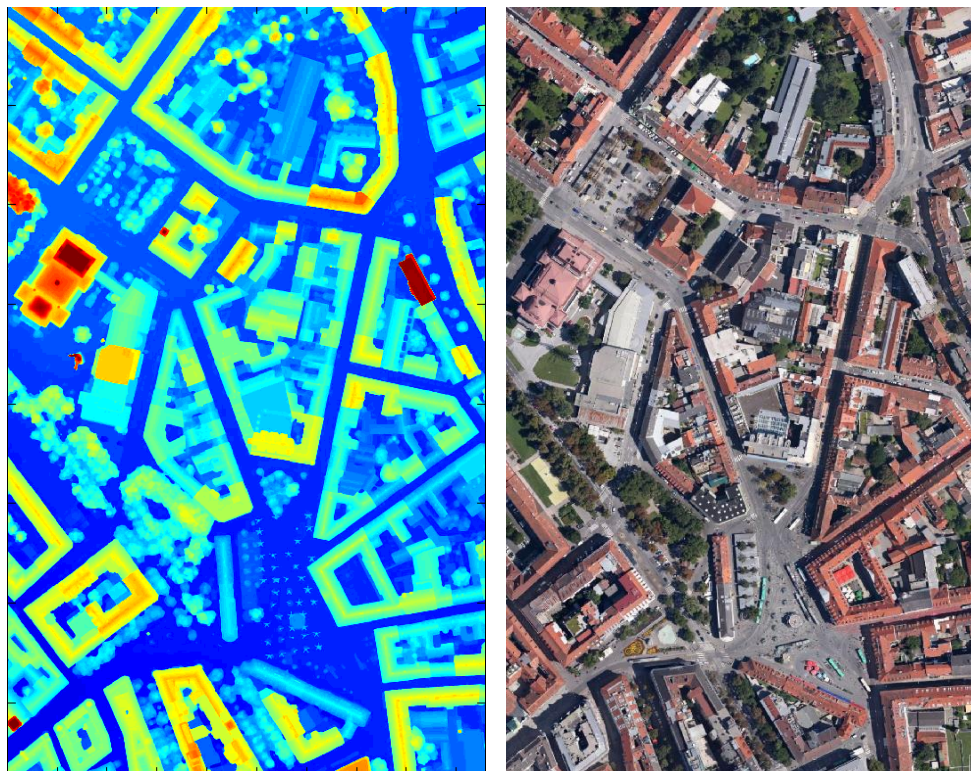
Figure 3.5 Digital Surface Model at 8 cm GSD (Left) and Aerial True Orthophoto at 30 cm GSD (Right); Location: Downtown Graz; [57, 59]
