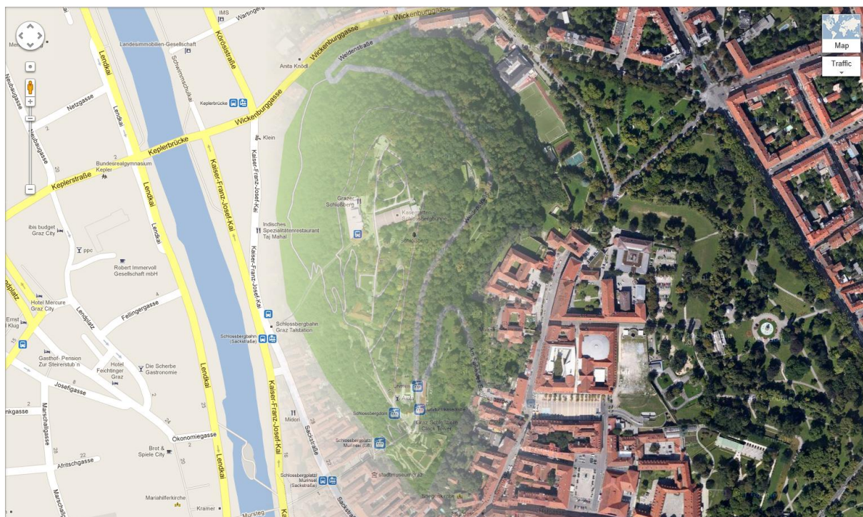
Figure 2.14 Comparison of Vector Data and Raster Data Used in Google Maps (Location: Schlossberg Mountain in Graz, Austria)
