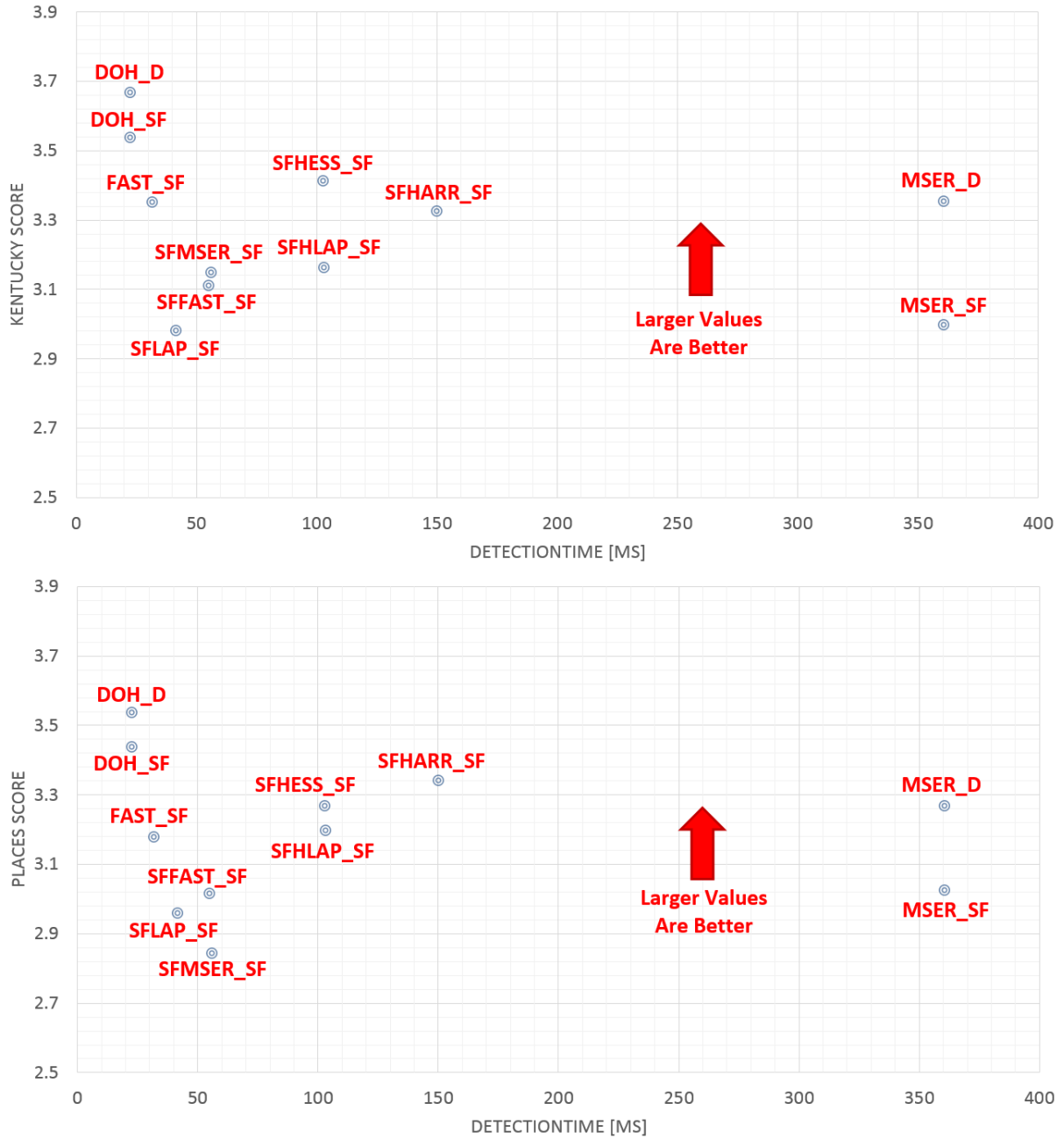
Figure 6.3 Comparison of Ranking Scores of Different Interest Point Detectors for Kentucky Dataset (Top) and Places Dataset (Bottom)
