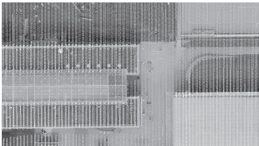
Figure 3.14 Comparison of UltraCam Aerial Photograph at 8 cm GSD with Superimposed Leica GeoSystems ALS50 LiDAR Point Cloud at 70 cm Spacing in Forward Direction and 45 cm across [170]
