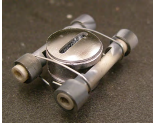
Figure 2.3: Tantalum crucible of the Cr electron bombardment evaporation source. The crucible is covered with a reusable molybdenum lid where the Cr atoms are emitted through the slit. The short ceramic tubes at the ends of the long tube prevent them from being coated with metal.
